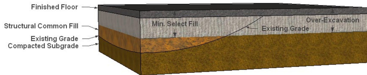
FIGURE 3.1: SELECT FILL PAD IMPROVEMENT
