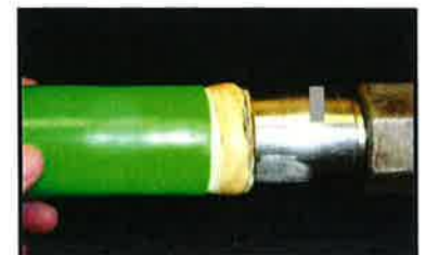
Flexible piping is bulging
