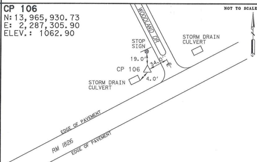
THE SURVEY CONTROL INFORMATION HAS BEEN ACCEPTED AND INCORPORATED INTO THIS PS&E
