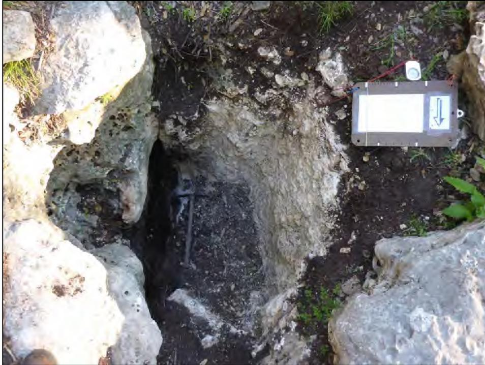
Figure 36. Feature AV12/X7 after excavation. Note the soil filled fracture potentially continuing downward. The fracture narrows downward and further excavation was not justified.
