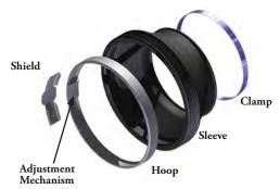
**Sleeve:** The heart of the boot connector, the sleeve, is designed for flexibility in all dimensions to accept relative movement between the pipe and the structure. Sleeves are manufactured, as standard, in EPDM which provides for protection against ultra-violet degradation while the structure is being stored and/or installed. Optionally, the sleeve is available in Nitrile for use in applications requiring oil-resistance. Sleeves are designed for use with either single or dual take-up clamps.
