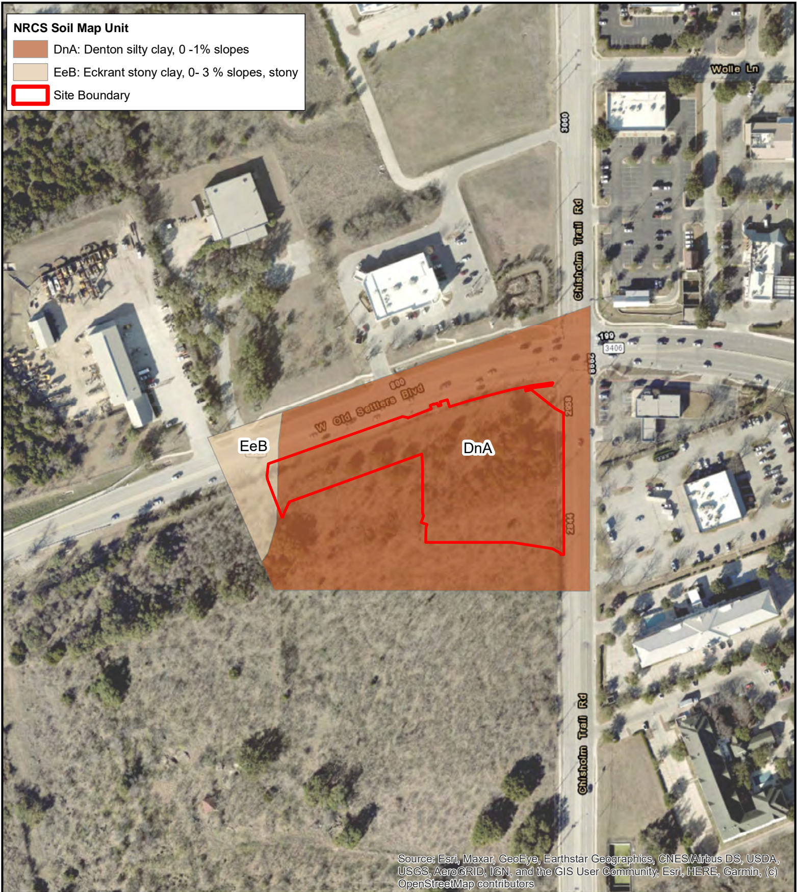
Fig.2 Site Soils Map QuikTrip Store #4166 SWC of Old Settler's & Chisholm Trail Round Rock, TX 78681
