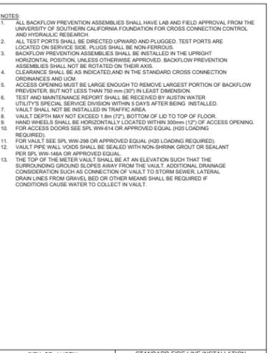
**STANDARD FIRE LINE INSTALLATION WITH MASTER METER**
