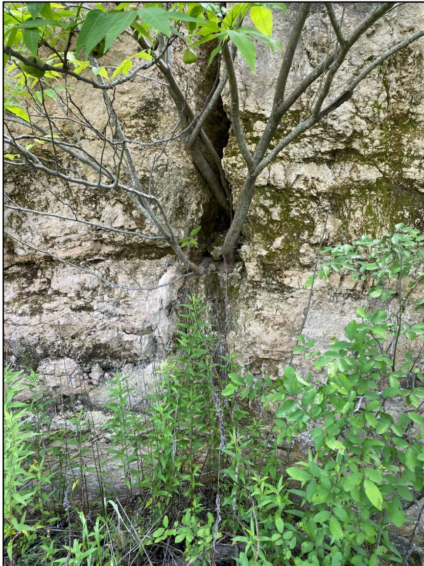
Feature Photo MPS-23 Solution Enlarged Fracture (Photo 2 of 2). The fracture was enlarged from chemical dissolution and physical (tree root growth) processes.
