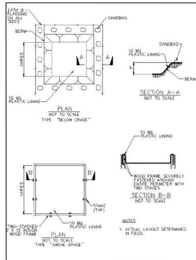
Temporary Concrete Washout Area Detail
