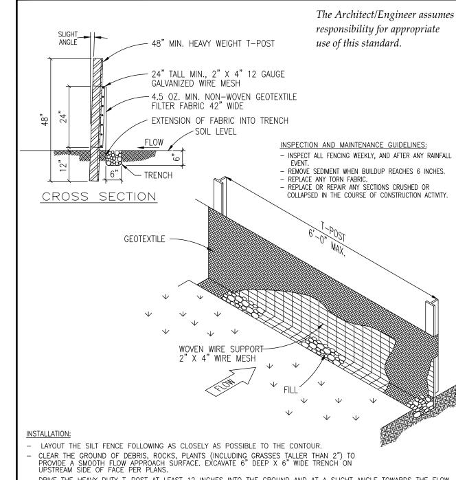
DRIVE THE HEAVY DUTY T-POST AT LEAST 12 INCHES INTO THE GROUND AND AT A SLIGHT ANGLE TOWARDS THE FLOW. ATTACH THE 2" X 4" 12 GAUGE WELDED WIRE MESH TO THE T-POST WITH 11 1/2 GAUGE GALVANIZED T-POST CLIPS. THE TOP OF THE WIRE TO BE 24" ABOVE GROUND LEVEL. THE WELDED WIRE MESH TO BE OVERLAPPED 6" AND
