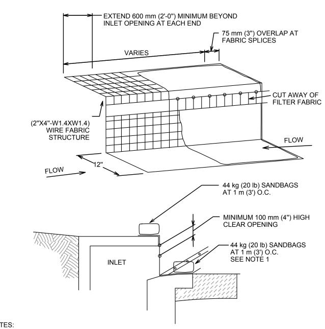
1. WHERE MINIMUM CLEARANCES CAUSE TRAFFIC TO DRIVE IN THE GUTTER, THE CONTRACTOR MAY SUBSITITUTE A 25 mm X 100 mm (1" X 4") BOARD SECURED WITH CONCRETE NAILS 1 m (3') O.C. NAILED INTO THE GUTTER IN LIEU OF SANDBAGS TO HOLD THE FILTER DIKÈ IN PLACE. UPON REMOVAL, CLEAN ANY DIRT/DEBRIS FROM NAILING LOCATIONS, APPLY CHEMICAL SANDING AGENT AND APPLY NON-SHRINK GROUT FLUSH WITH SURFACE
