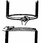
Carefully clean all dirt & foreign objects from the joining surface of the bell or groove end of pipe.
