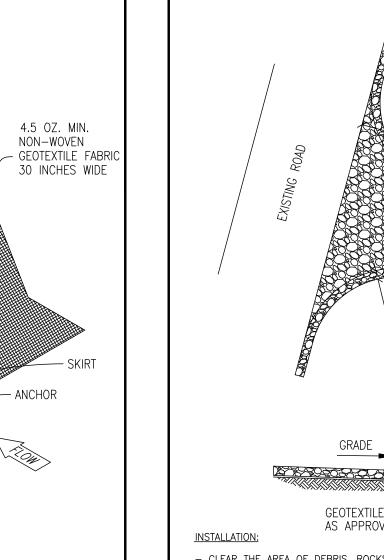
LAYOUT THE FILTER DIKE FOLLOWING AS CLOSELY AS POSSIBLE TO THE CONTOUR. CLEAR THE GROUND OF DEBRIS, ROCKS OR PLANTS THAT WILL INTERFERE WITH INSTALLATION. PLACE THE FILTER DIKE SECTIONS ONE AT A TIME, WITH THE SKIRT ON THE UPHILL SIDE TOWARDS THE DIRECTION OF FLOW, ANCHORING EACH SECTION TO THE GROUND BEFORE THE NEXT SECTION IS PLACED.
