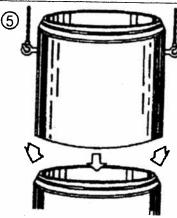
Align the bell & spigot to be joined. Before homing the joint, check that the gasket is in contact with the bell end entrance taper around the entire circumference.
