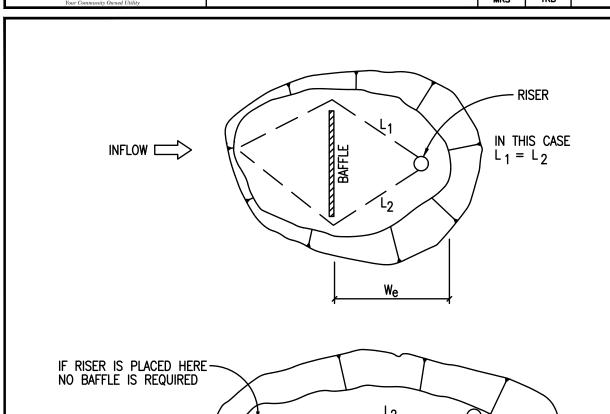
SEDIMENT BASIN BAFFLE DESIGN  $W_e = A / (L_1 + L_2)$
