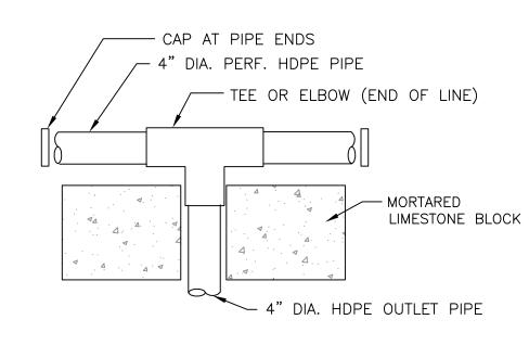
SUBDRAIN PIPE OUTLET DETAIL N.T.S.
