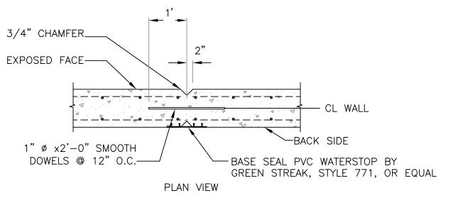
NOTE: CONTRACTION JOINT SPACING NOT TO EXCEED 20'-0" AND AT ALL ABRUPT CHANGES IN WALL HEIGHT.
