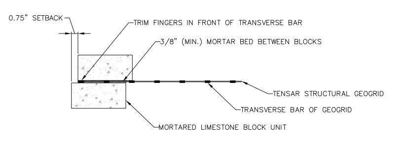
NATURAL LIMESTONE BLOCK TO GEOGRID CONNECTION DETAIL N.T.S.
