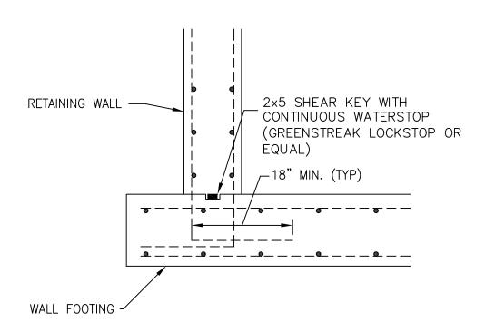
RETAINING WALL BASE JOINT AND WATERSTOP DETAIL
