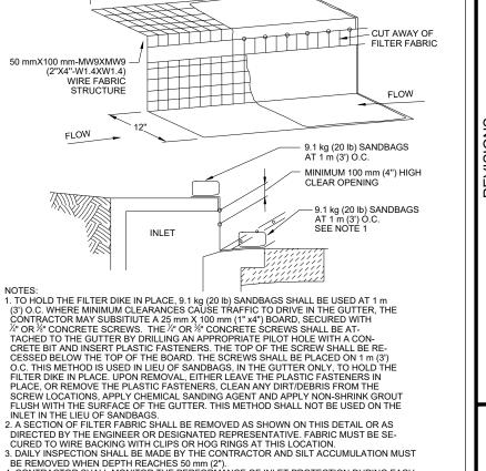
3. DAILY INSPECTION SHALL BE MADE BY THE CONTRACTOR AND SILT ACCUMULATION MUST BE REMOVED WHEN DEPTH REACHES 50 mm (2"). 4. CONTRACTOR SHALL MONITOR THE PERFORMANCE OF INLET PROTECTION DURING EACH RAINFALL EVENT AND IMMEDIATELY REMOVE THE INLET PROTECTIONS IF THE STORM-WATER BEGINS TO OVERTOP THE CURB.
