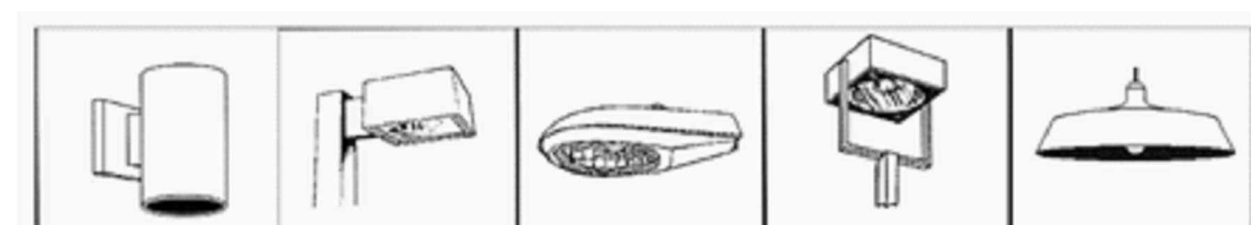
Figure 34: Examples of fully-shielded light fixtures.
