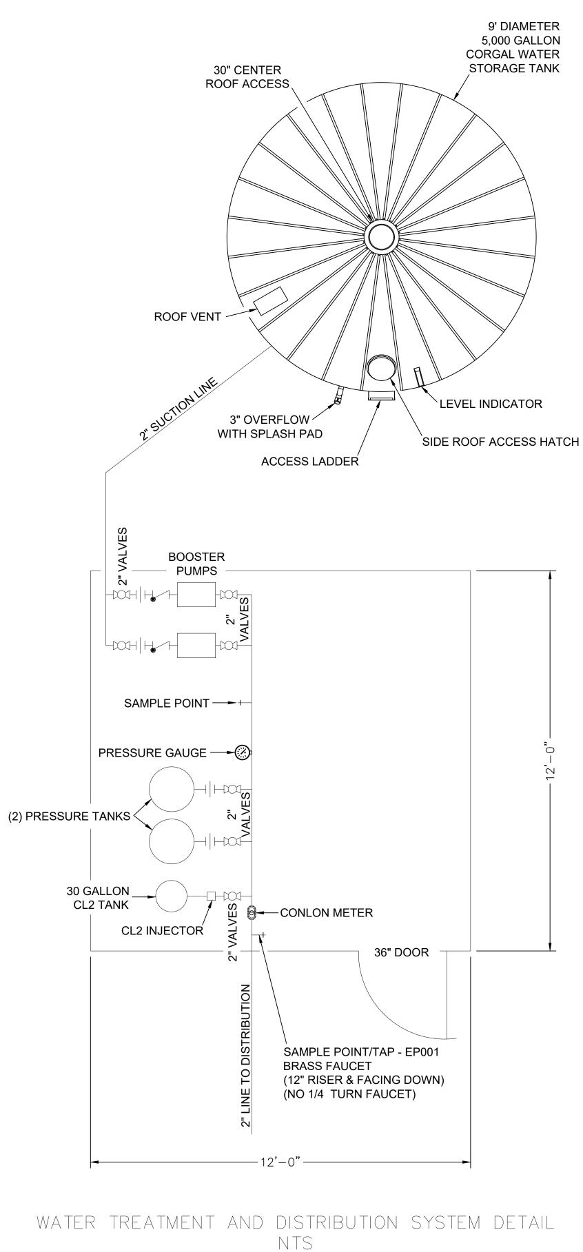
NOTE: WELL, TREATMENT AND DISTRIBUTION SYSTEM ARE TO BE ENCLOSED IN INTRUDER RESISTANT FENCE OR OTHER APPROVED INTRUDER RESISTANT MECHANISM
