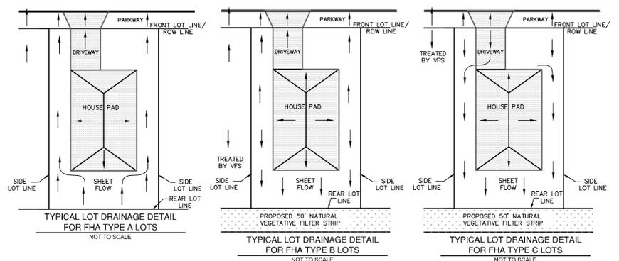
NOTE: ROOF DRAINAGE PATTERN IS APPROXIMATE AND SUBJECT TO CHANGE BASED ON FINAL HOUSE PAD DESIGN. HOWEVER RUNOFF FROM DRIVEWAY, ROOF OR OTHER IMPERVIOUS SURFACES WITHIN THE LOT WILL NOT FLOW ACROSS MORE THAN 72" OF IMPERVIOUS SURFACE BEFORE REACHING THE PROPOSED 50' NATURAL VEGETATIVE FILTER STRIP. FINAL LOT GRADING TO ALLOW FOR SHEET FLOW OVER VEGETATIVE FILTER STRIP.
