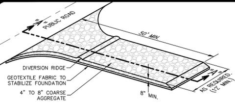
**SCHEMATIC OF TEMPORARY CONSTRUCTION ENTRANCE/EXIT**
