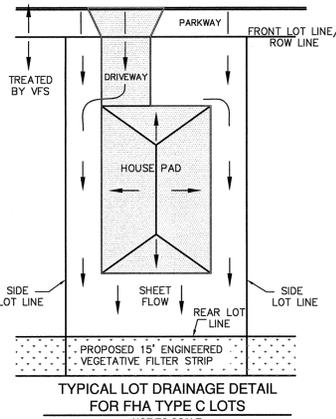
NOTE: ROOF DRAINAGE PATTERN IS APPROXIMATE AND SUBJECT TO CHANGE BASED ON FINAL HOUSE PAD DESIGN. HOWEVER RUNOFF FROM DRIVEWAY, ROOF OR OTHER IMPERVIOUS SURFACES WITHIN THE LOT WILL NOT FLOW ACROSS MORE THAN 72" OF IMPERVIOUS SURFACE BEFORE REACHING THE PROPOSED 15' ENGINEERED VEGETATIVE FILTER STRIP. FINAL LOT GRADING TO ALLOW FOR SHEET FLOW OVER VEGETATIVE FILTER STRIP.
