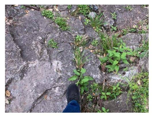
**Photo 08.** Feature BC-03. Zone extends approximately 50 feet within a drainage ditch constructed in exposed Edwards limestone. Average aperture 1 inch and average trend is 30 degrees. Infill with soft mud and fine packed sediments.
