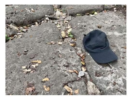
**Photo 10.** Feature BC-04. Solution-enlarged fracture zone. Coordinates: -97.85384, 30.2374. Average aperture 1-4 inches and fractures trend between 130-150 degrees. Infill with cobbles, pebbles, and fine packed soil.
