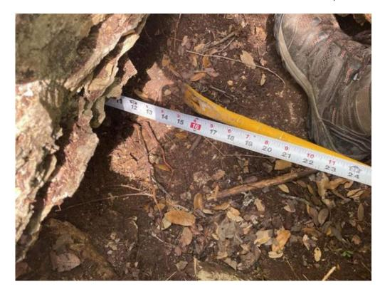
**Photo 02.** Feature BC-01 post excavation. Bedrock encountered at 4 feet below surface. Extends northwest approximately 1 foot laterally along solution enlarged bedding plane in subsurface. Terminates into hard-packed soil.
