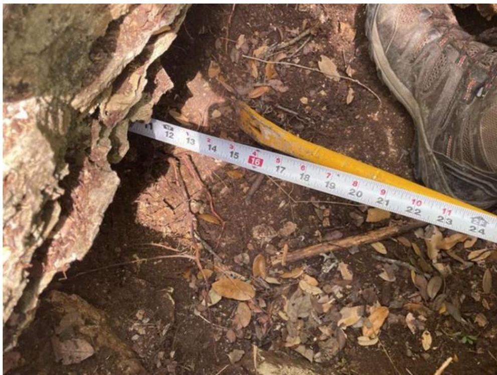
**Photo 02.** Feature BC-01 post excavation. Bedrock encountered at 4 feet below surface. Extends northwest approximately 1 foot laterally along solution enlarged bedding plane in subsurface. Terminates into hard-packed soil.
