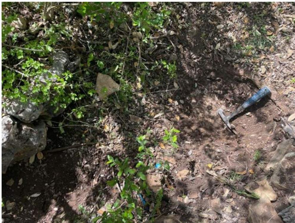
**Photo 13.** Feature BC-05. After excavation. Feature determined to be non-karst closed depression and terminates into bedrock with no aperture or voids into subsurface.
