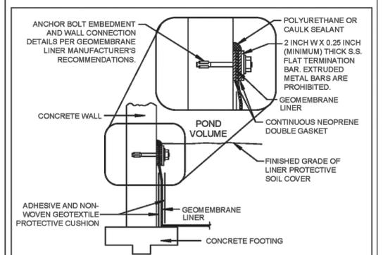
**CONCRETE WALL GEOMEMBRANE LINER ATTACHMENT**
