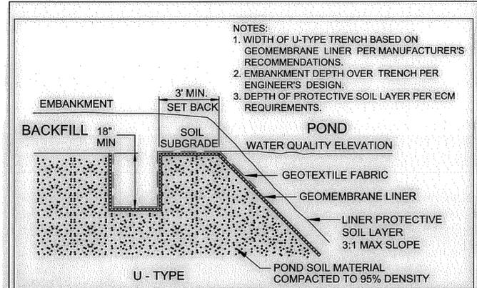
**ANCHOR TRENCHES FOR GEOMEMBRANE LINERS**
