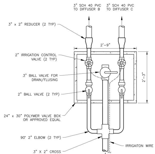
**SECONDARY VALVE BOX DETAIL (C)**
