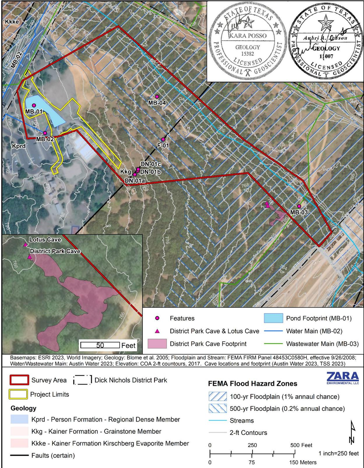
Figure 3. Geology of the Dick Nichols District Park Water Quality Retrofit Survey Area with the locations of all features identified during the field survey.
