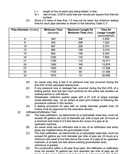
hours at the same minimum test head as in subparagraph (C) of this If the quantity of infiltration or exfiltration exceeds the maximum quantity specified, an owner shall undertake remedial action in order to reduce
