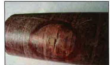
Fiberglass piping is cracked
