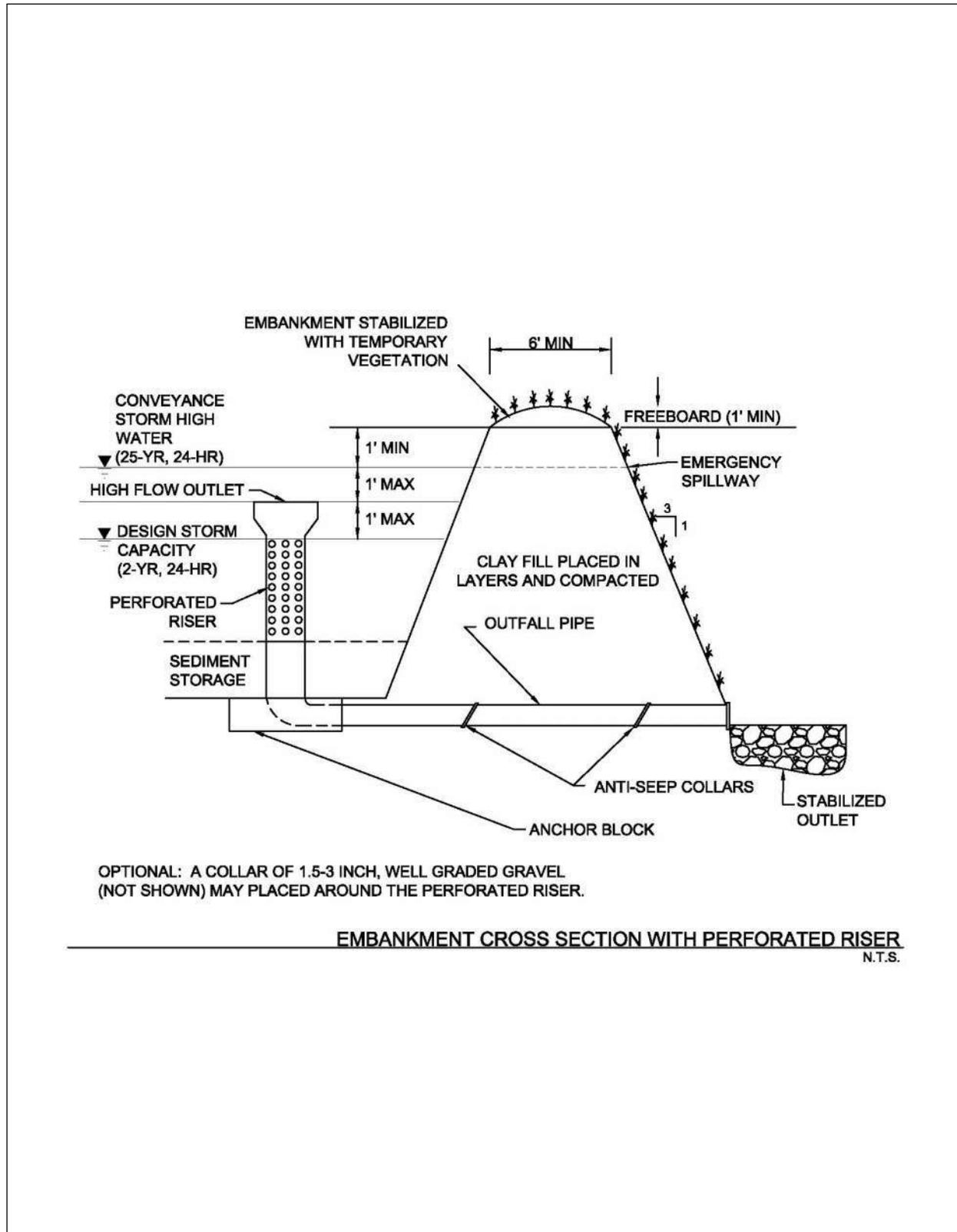
Figure 3.22 Schematic of Basin Embankment with Perforated Riser
