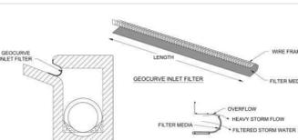
**CROSS-SECTION SHOWING PLACEMENT OF GEOSOLUTIONS CURB INLET**
