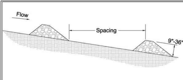
**Description:** Check dams are small barriers consisting of loose rock, rock bags, or organic filter tubes placed across a drainage swale or ditch. They reduce the velocity of small concentrated flows, provide a limited barrier for sediment and reduce the potential for erosion of the swale or ditch.
