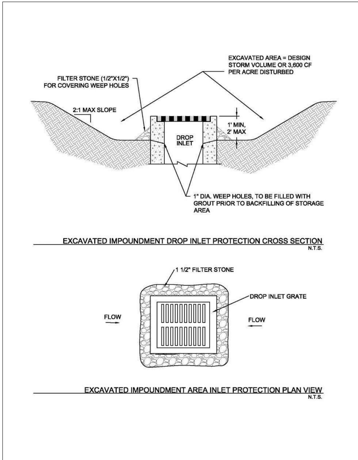
**Figure 3.11 Schematics of Excavated Impoundment Area Inlet Protection**
