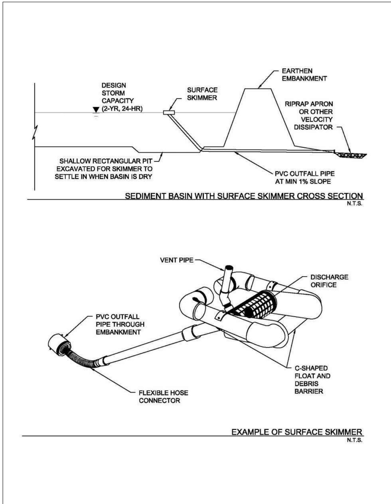
**Figure 3.19 Schematics of Sediment Basin with Surface Skimmer**
