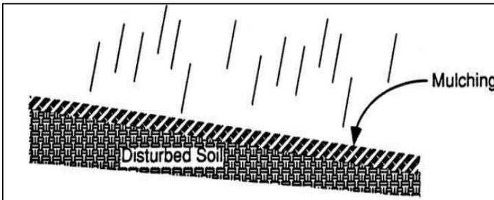
**Description:** Mulching is the application of a uniform layer of organic material over barren areas to reduce the effects of erosion from rainfall. Types of mulch include compost mixtures, straw, wood chips, bark, or other fibers. Commercialized surface treatments that combine straw or other mulch material with organic or inorganic soil binding systems are also available and are particularly useful on steep slopes.
