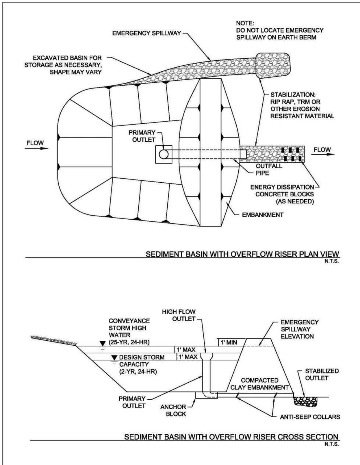
Figure 3.20 Schematics of Sediment Basin with Overflow Riser
