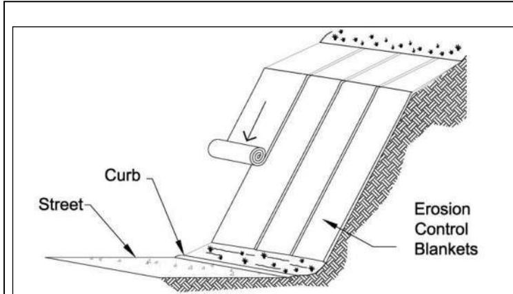
**Description:** An erosion control blanket (ECB) is a temporary, degradable, rolled erosion control product that reduces soil erosion and assists in the establishment and growth of vegetation. ECBs, also known as soil retention blankets, are manufactured by many companies and are composed primarily of processed, natural, organic materials that are woven, glued, or structurally bound together with natural fiber netting or mesh on one or both sides.
