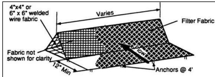
**Description:** A triangular sediment filter dike is a self-contained silt fence consisting of filter fabric wrapped around welded wire fabric and shaped into a triangular cross section. While similar in use to a silt fence, the dike is reusable, sturdier, transportable, and can be used on paved areas or in situations where it is impractical to install embedded posts for support.
