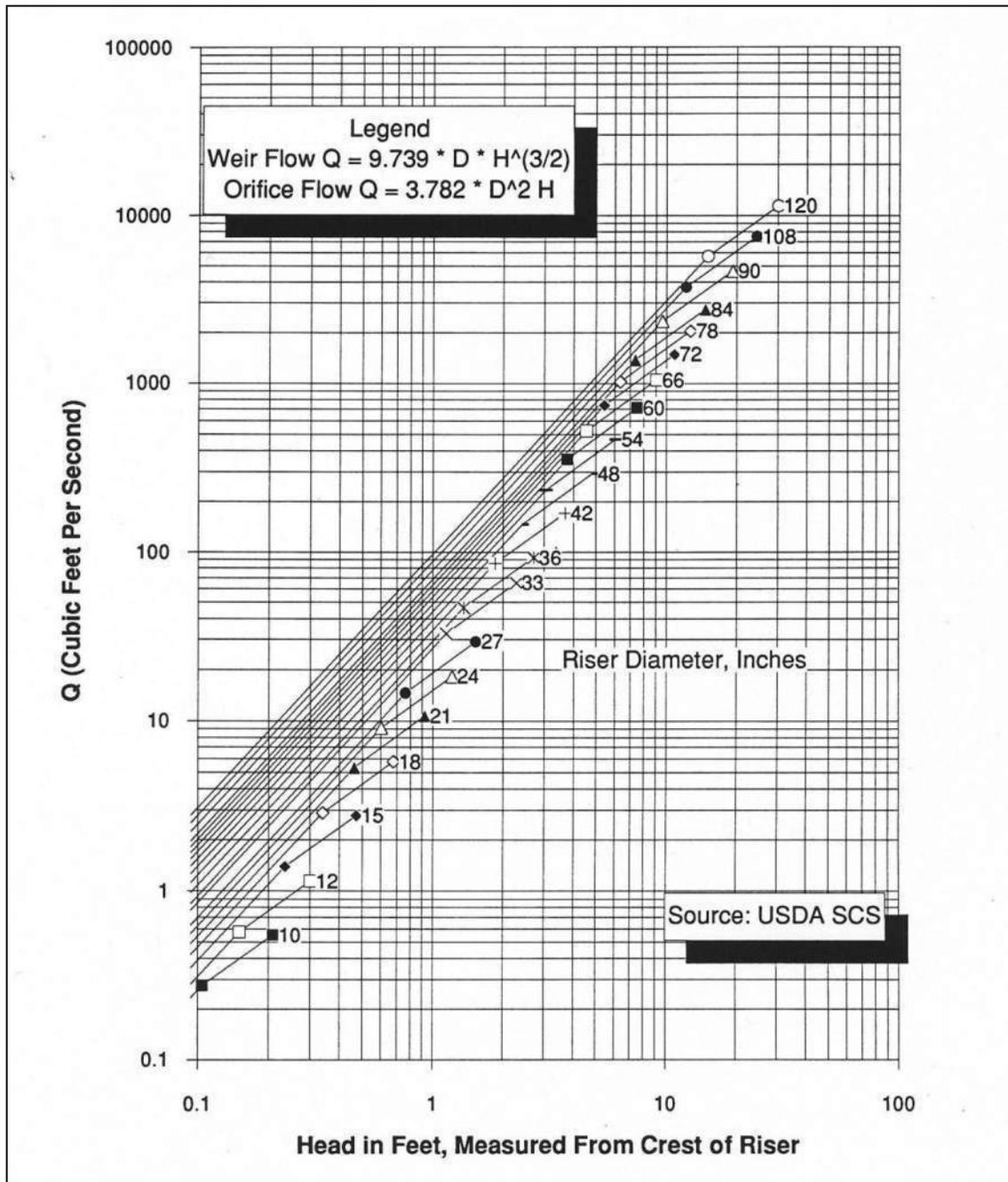
Figure 3.24 Riser Inflow Curves for Basin Outlet Design
