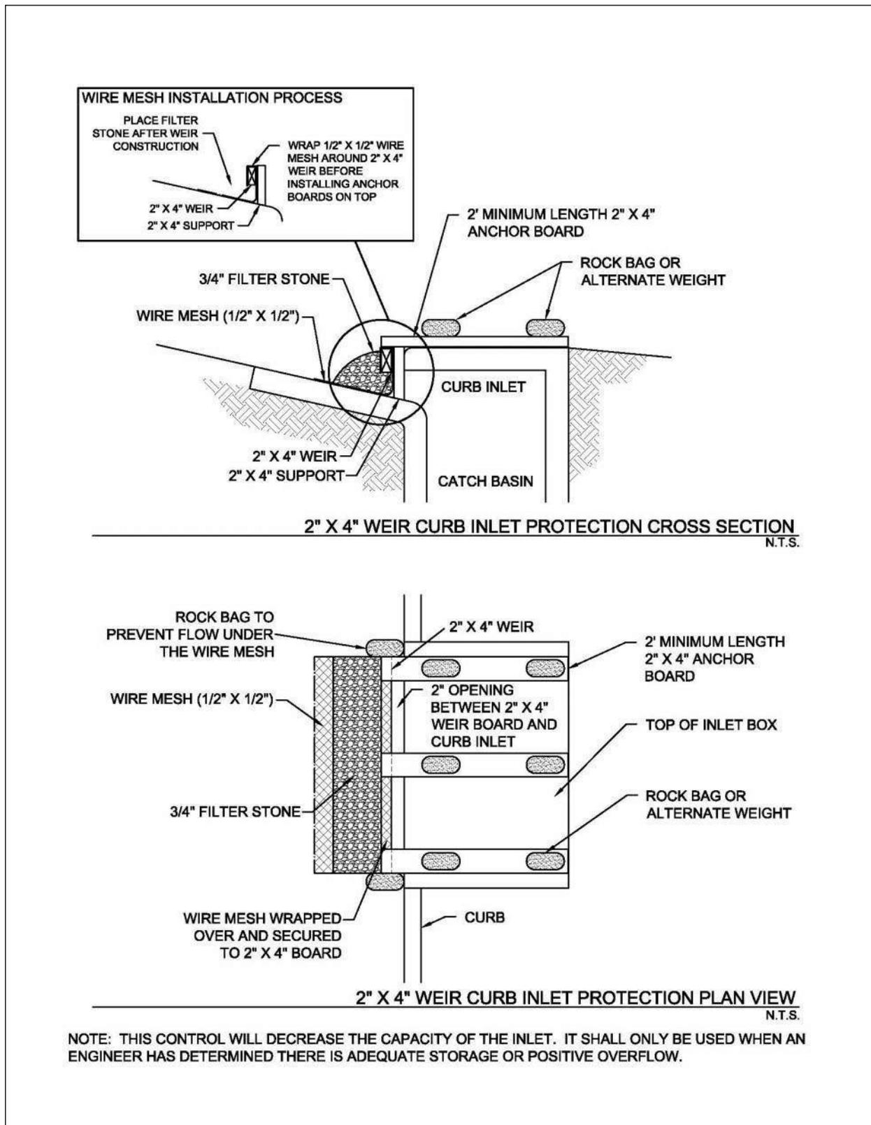
**Figure 3.5 Schematics of 2"x4" Weir Curb Inlet Protection**
