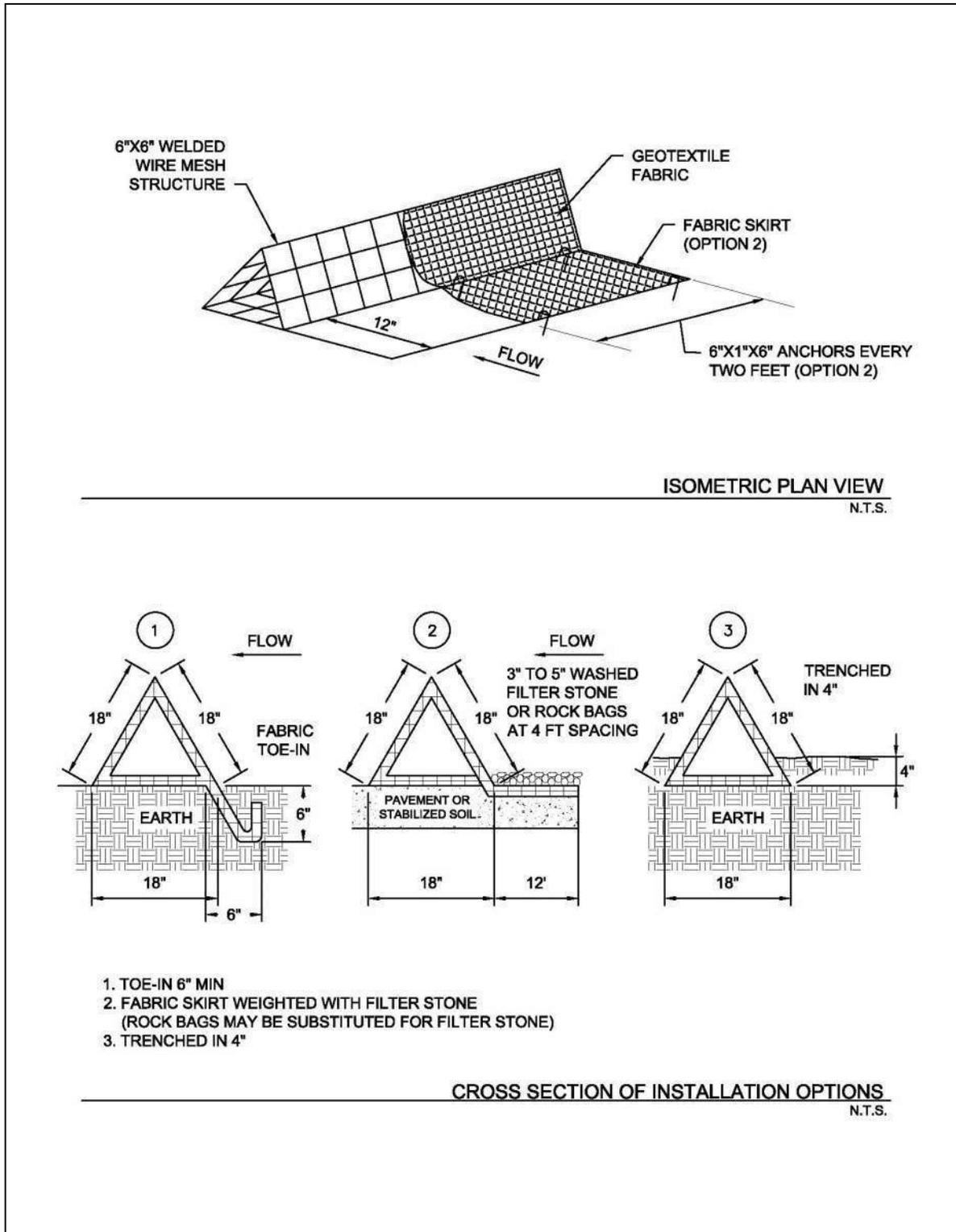
Figure 3.32 Schematics of Triangular Sediment Filter Dike
