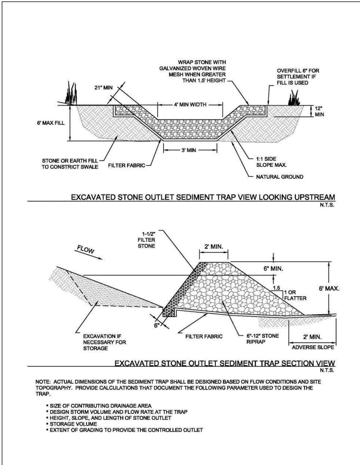
**Figure 3.30 Schematics of Excavated Stone Outlet Sediment Trap**
