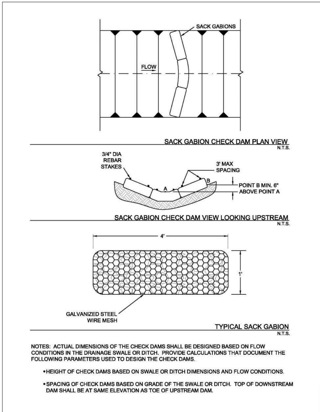
**Figure 2.3 Schematics of Sack Gabion Check Dams**
