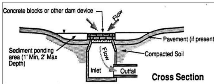
**Description:** Inlet protection consists of a variety of methods to intercept sediment at low point inlets through the use of depressed grading, filter stone, filter fabric, inlet inserts, organic filter tubes and other materials. The protection devices are placed around or across the inlet openings to provide localized detention or filtration of sediment and floatable materials in stormwater. Protection devices may be assembled onsite or purchased as manufactured assemblies.
