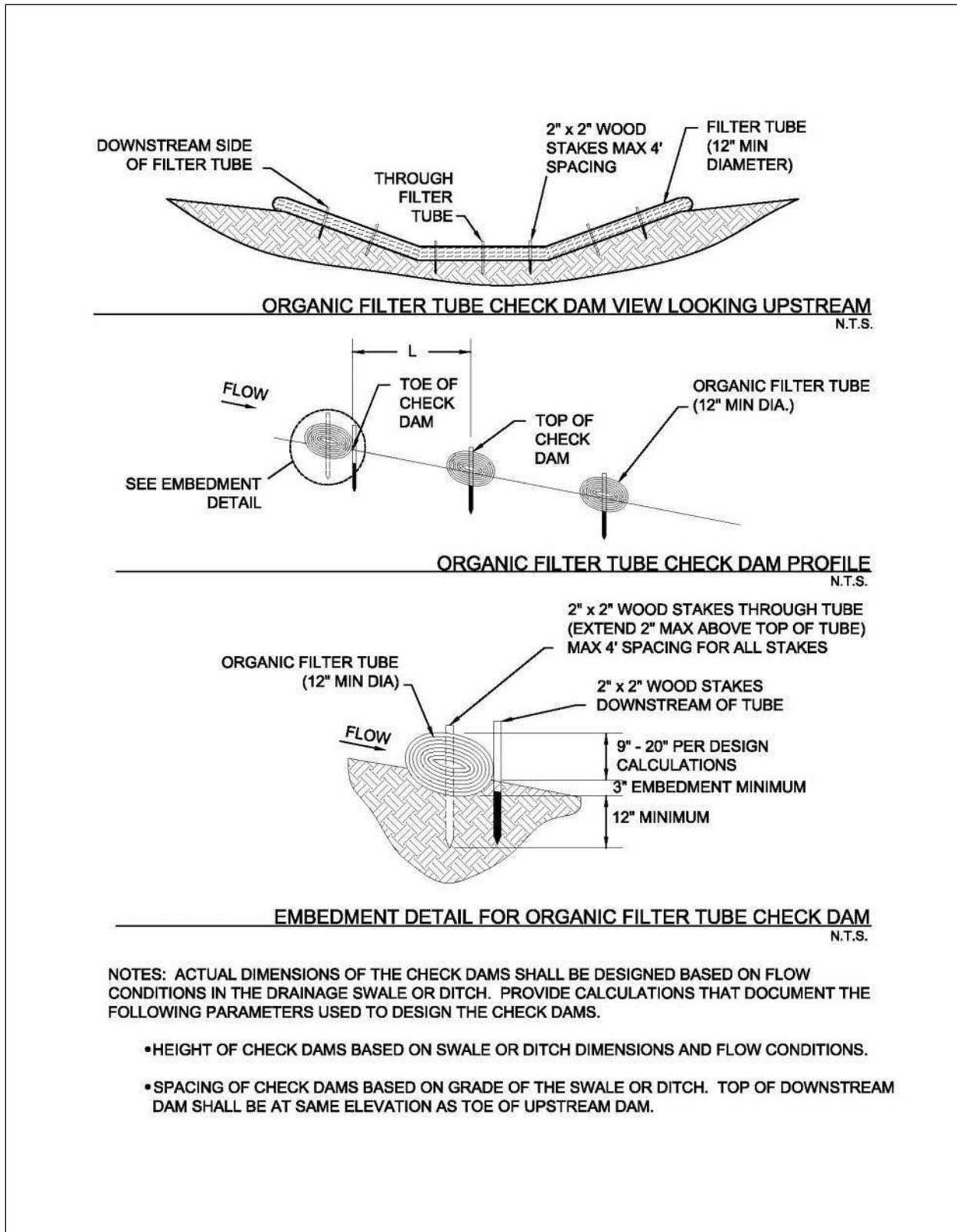
**Figure 2.4 Schematics of Organic Filter Tube Check Dams**
