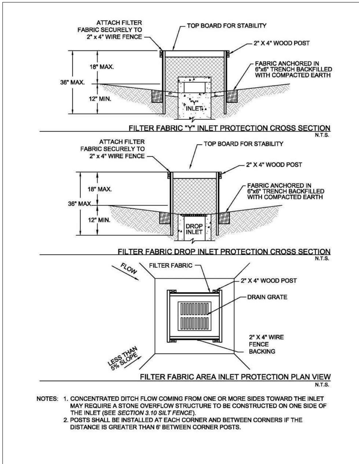
**Figure 3.10 Schematics of Filter Fabric Area Inlet Protection**
