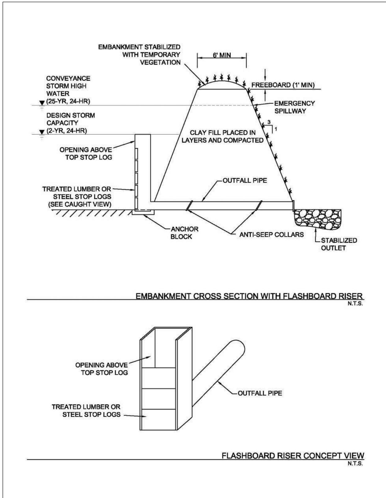
**Figure 3.21 Schematics of Basin Embankment with Flashboard Riser**
