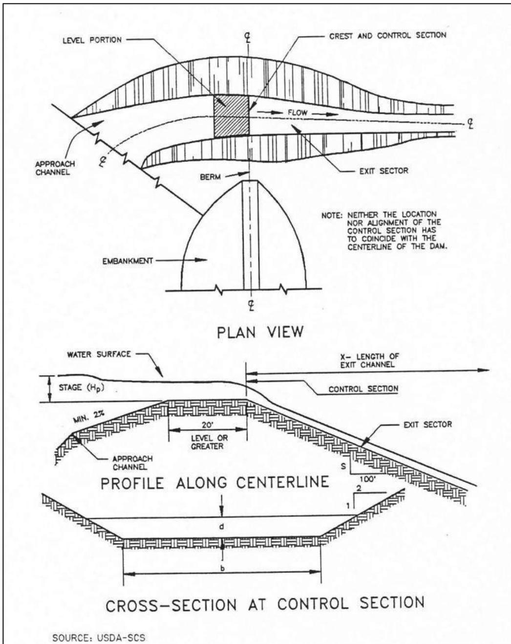
Figure 3.25 Example of Excavated Earth Spillway Design
