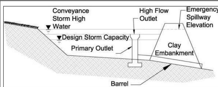
**Description:** A sediment basin is an embankment with a controlled outlet that detains stormwater runoff, resulting in the settling of suspended sediment. The basin provides treatment for the runoff as well as detention and controlled release of runoff, decreasing erosion and flood impacts downstream.
