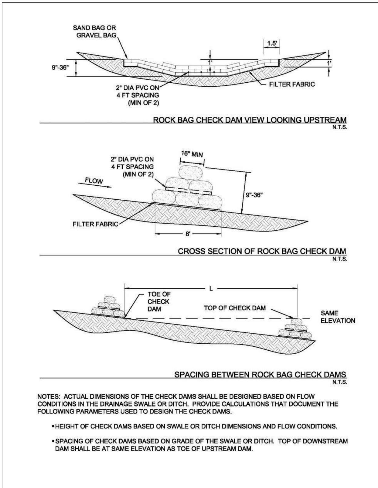
Figure 2.2 Schematics of Rock Bag Check Dams
