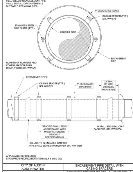
ENCASEMENT PIPE DETAIL WITH CASING SPACERS
