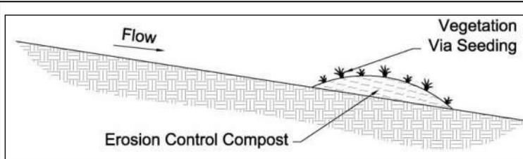
**Description:** Organic filter berms, also called compost filter berms, are linear berms constructed of a mix of compost and wood chips. They are placed on a contour to control runoff. The organic filter berm provides both filtration and time for sediment settling by reducing the velocity of the runoff.
