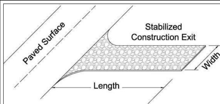
**Description:** A stabilized construction exit is a pad of crushed stone, recycled concrete or other rock material placed on geotextile filter cloth to dislodge soil and other debris from construction equipment and vehicle tires prior to exiting the construction site. The object is to minimize the tracking of soil onto public roadways where it will be suspended by stormwater runoff.
