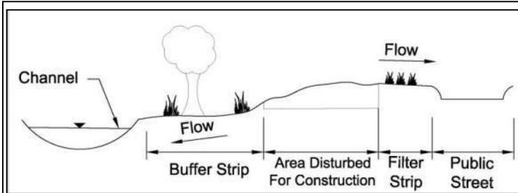
**Description:** Buffer strips (existing vegetation) and filter strips (planted vegetation) are sections of vegetated land adjacent to disturbed areas. They are designed with low slopes to convey sheet flow runoff from disturbed areas, resulting in the removal of sediment and other pollutants as the runoff passes through vegetation and infiltration occurs.
