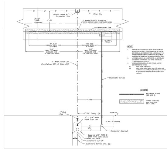
TYPICAL DOUBLE WATER/WASTEWATER SERVICE - PLAN
