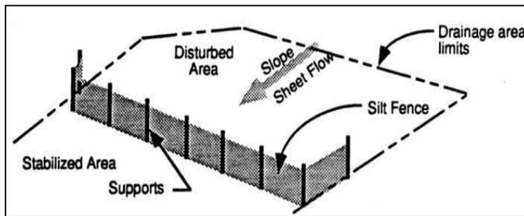
**Description:** A silt fence consists of geotextile fabric supported by wire mesh netting or other backing stretched between metal posts with the lower edge of the fabric securely embedded six-inches in the soil. The fence is typically located downstream of disturbed areas to intercept runoff in the form of sheet flow. A silt fence provides both filtration and time for sediment settling by reducing the velocity of the runoff.
