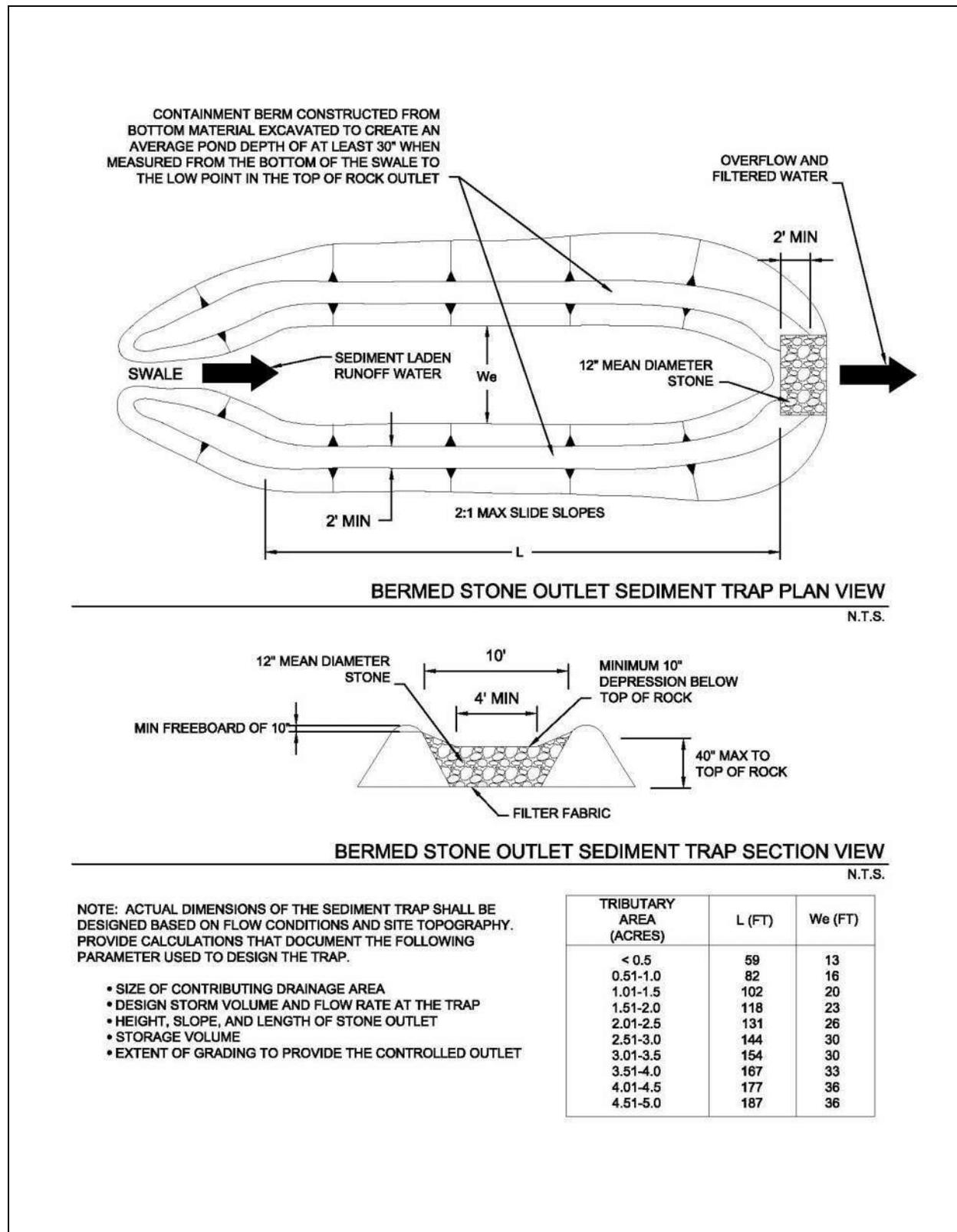
**Figure 3.31 Schematics of Bermed Stone Outlet Sediment Trap**
