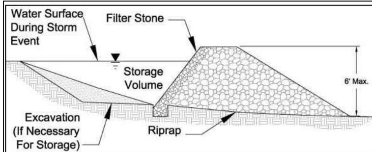
**Description:** A stone outlet sediment trap is a small detention area formed by placing a stone embankment with an integral stone filter outlet across a drainage swale for the purpose of detaining sediment-laden runoff from construction activities. The sediment trap detains runoff long enough to allow most of the suspended sediment to settle while still allowing for diffused flow of runoff.
