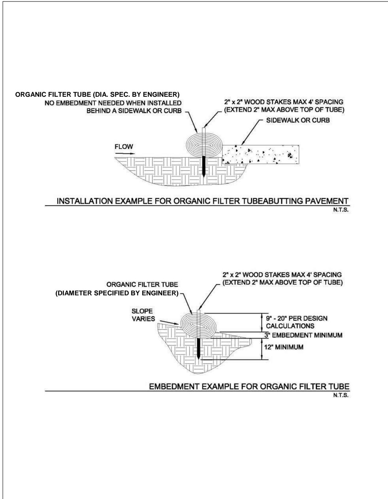
**Figure 3.16 Examples of Organic Filter Tube Installation Methods**
