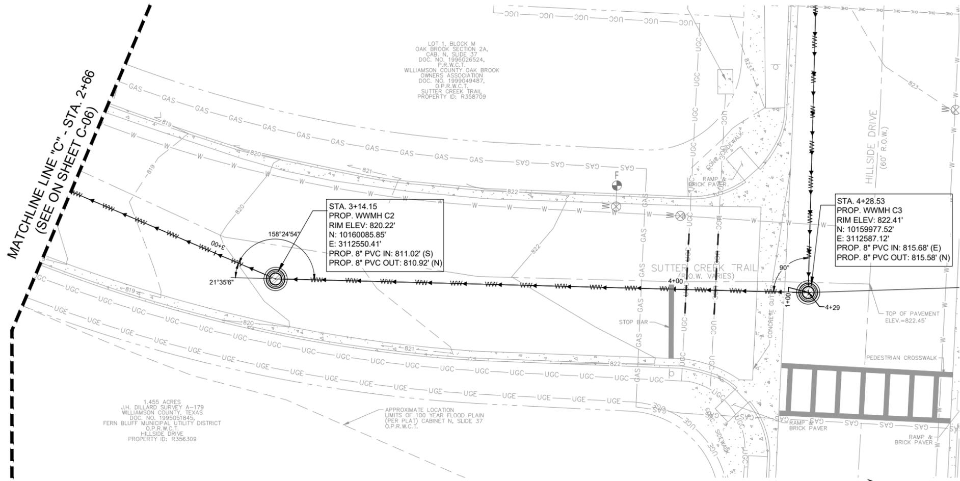
**SUTTER CREEK TRAIL WASTEWATER LINE "C" PLAN STA. 2+66 TO 4+32.83**
