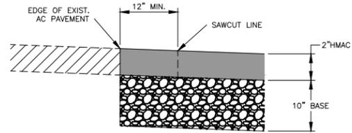
1 SAWCUT PAVEMENT CONFORM DETAIL (CAT HOLLOW)
