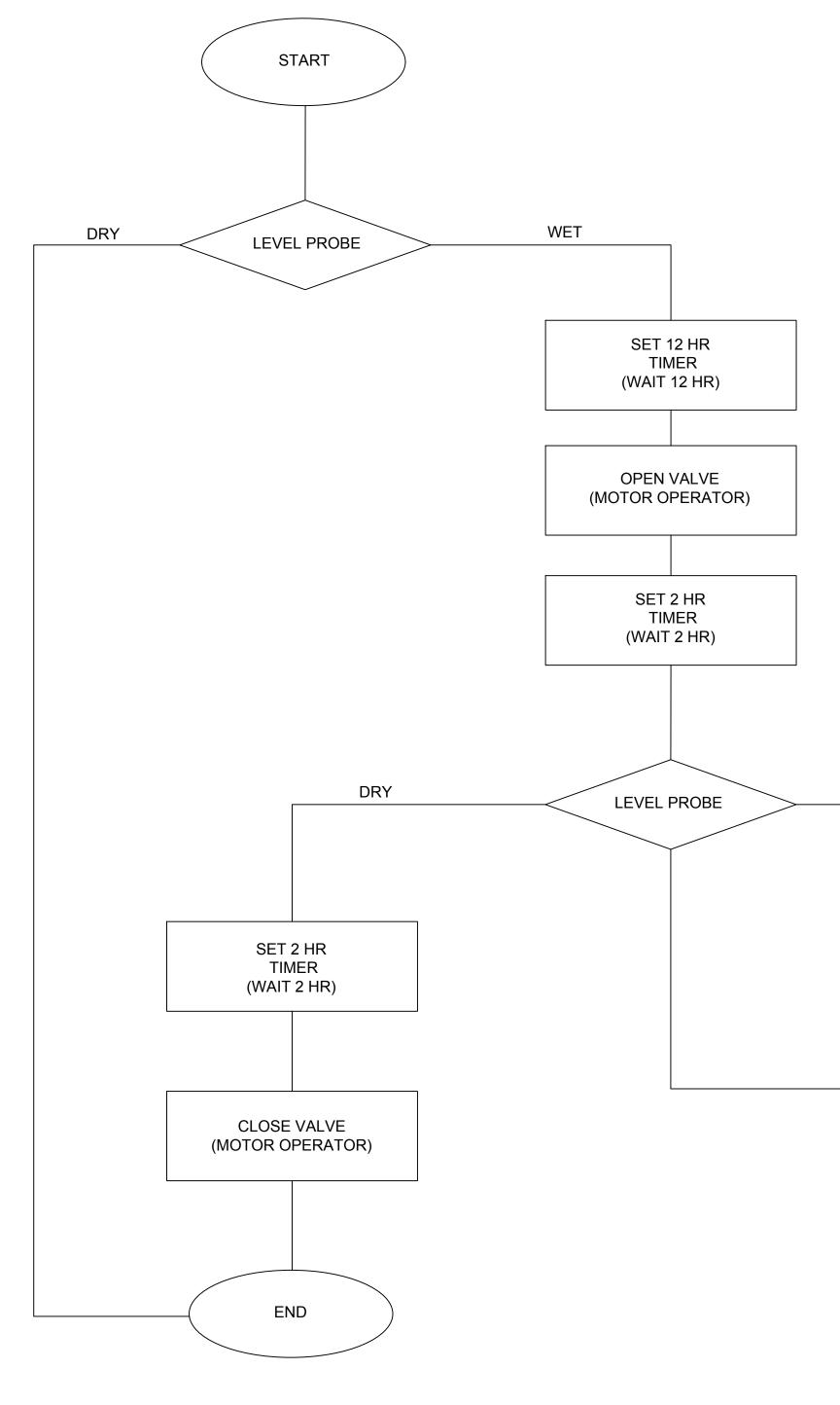
POND LEVEL CONTROL FLOW DIAGRAM NTS
