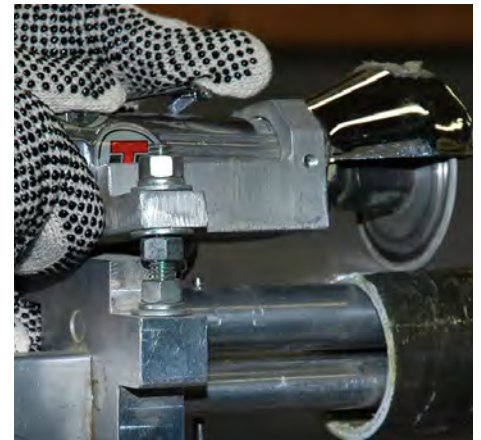
Jacket Cutter Tool - Cuts containment jacket from 2"-4" Dualoy 3000/LCX pipe
