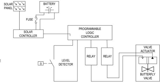
STORMWATER MANAGEMENT POND FLOW CONTROL RELEASE VALVE CIRCUIT DIAGRAM
