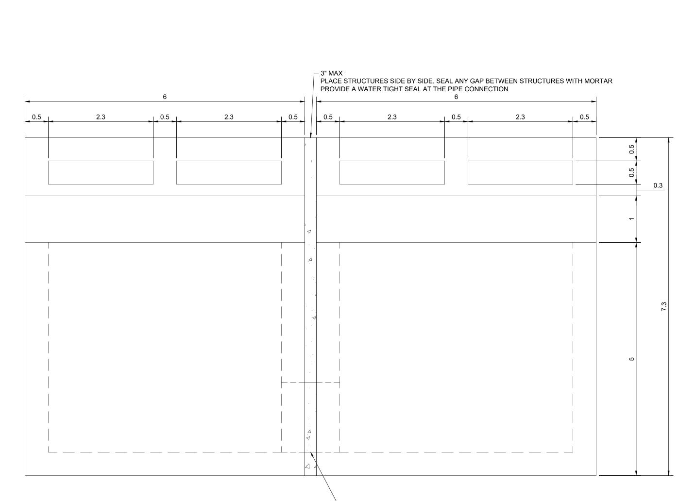
CONNECT 2 - 5' PCU INLETS WITH 18" RCP TO FORM FULL DEPTH 10' INLET
