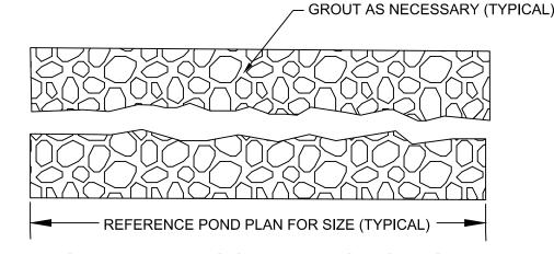
PLACE RIP-RAP AND LEAN GROUT IN ALL AREAS INDICATED ON THE DRAWING. THE STONE SHALL CONSIST OF FIELD STONE OR ROUGH, PRACTICAL. THE STONES SHALL BE DENSE, RESISTANT TO THE ACTION OF AIR AND WATER, AND SUITABLE IN ALL ASPECTS FOR THE PURPOSE INTENDED, UNLESS OTHERWISE SPECIFIED, ALL STONES USED AS RIP-RAP SHALL WEIGH BETWEEN 2-4 POUNDS EACH, AND AT LEAST 60 PERCENT OF THE STONES SHALL WEIGH MORE THAN 3 POUNDS EACH.
