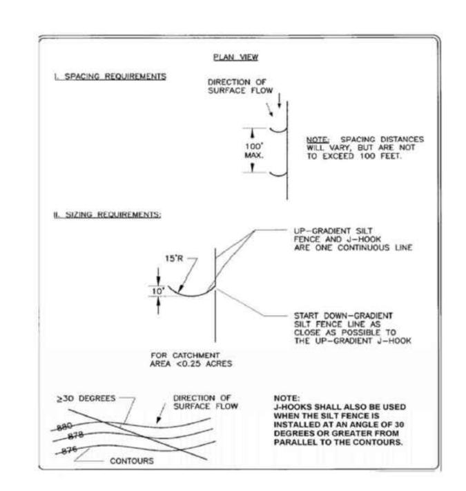
FIGURE 1.4.5.G.4 SILT FENCE J - HOOK DETAILS
