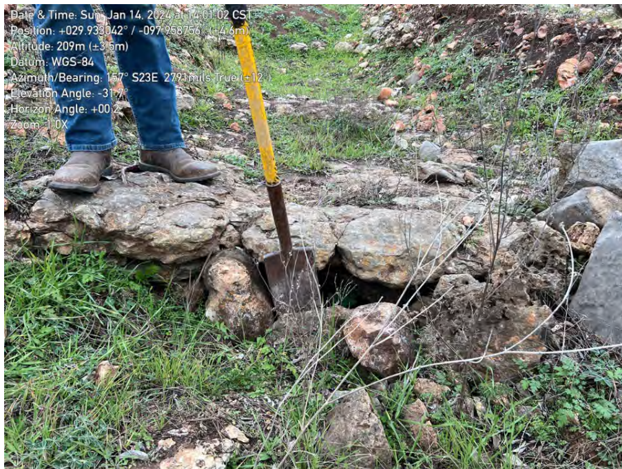
Photo 6: Feature S-06 Solution cavity/sinkhole. (N 29.933042° W -97.958756°)
