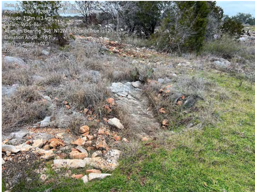
Photo 9: Feature S-9 Sinkhole within Fracture Rock Zone. (N 29.932887° W -97.958883°)
