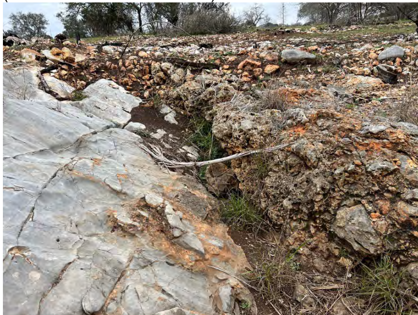
Photo 12 Feature S-12 Fracture Rock Zone with Dipping Beds and Geologic Contact (N 29.933056° W -97.958766°)
