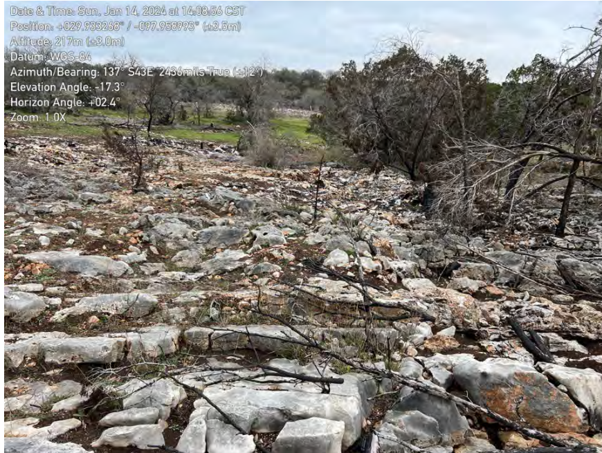
Photo 11 Fractured Rock Zone with Dipping Beds (N 29.933268° W -97.958993°)
