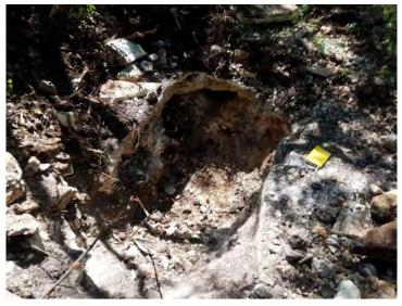
PHOTO 20 View of geologic feature F-17 (sinkhole) after mechanical excavation, facing down
