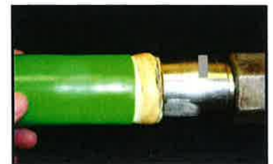
Flexible piping is bulging
