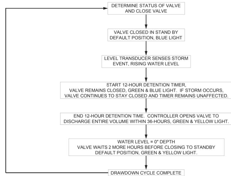
DETAIL 2 NOTE: LOGIC FLOW CHART FOR "TEST MODE" INCLUDED IN OPERATIONS AND MAINTENANCE MANUAL.
