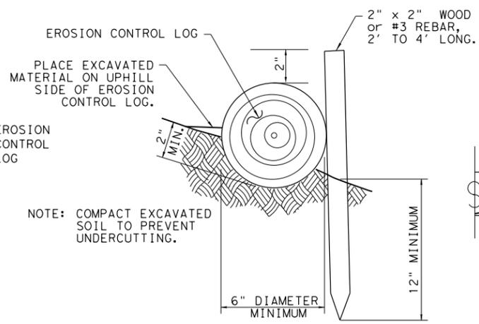
STAKE AND LASHING ANCHORING DETAIL
