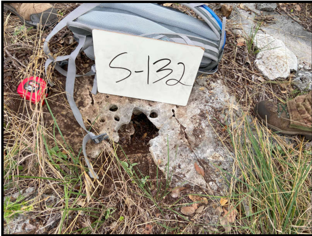
S-132: Solution cavity located on the northcentral part of the Site.
