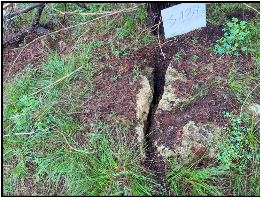
S-139: Solution-enlarged fracture located on the eastern part of the Site.
