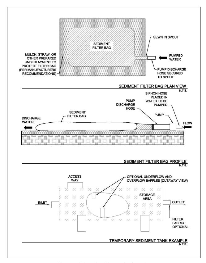
Figure 3.4 Schematics of Dewatering Controls
