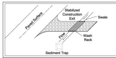
**Description:** Wheel cleaning systems are used with a stabilized construction exit to remove soil from vehicle wheels and undercarriages prior to leaving the construction site. The cleaning system may be as simple as uneven, steel racks that "rumble" the vehicle or as complex as a premanufactured wash bay. Systems that include wash water must provide for collecting the water and removing sediments and other pollutants prior to discharge.
