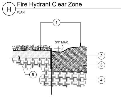
1. DIFFERENT PLANTING TREATMENTS. 2. METAL EDGING 3. BED SOIL. 12" MINIMUM DEPTH. REF: NOTES AND/OR SPECS FOR MIX. 4. NATIVE SOIL 5. 4" TOPSOIL. REF: NOTES AND/OR SPECS FOR MIX. & DEPTH.
