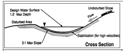
**Description:** An interceptor swale is a small v-shaped, trapezoidal, or parabolic channel that collects runoff and directs it to a desired location. It can either have a natural grass lining or, depending on slope and design velocity, a protective lining of erosion control blankets, turf reinforcement mats, or rock riprap.
