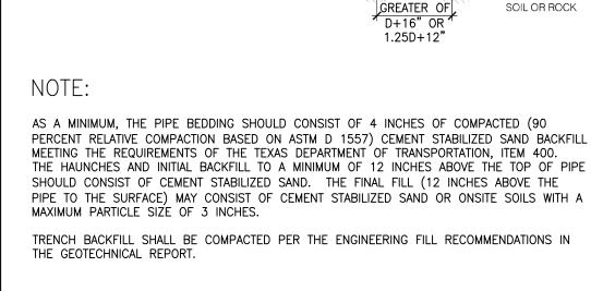
UTILITY TRENCHES SHOULD NOT BE CONSTRUCTED WITHIN A ZONE DEFINED BY A LINE THAT
