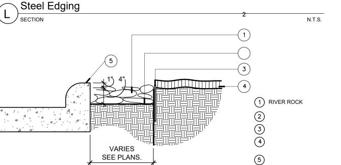
RIVER ROCK TO BE SMOOTH & ROUND. BETWEEN 2"-3" IN <u>SECTION</u> SIZE, COLOR: VARYING SHADES OF TAN/BROWN. SUBMIT PHOTO SAMPLE TO ARCHITECT / ENGINEER FOR APPROVAL River Rock SECTION N.T.S.
