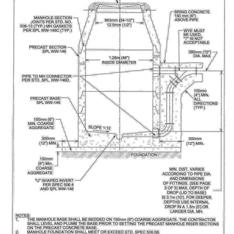
PRECAST MANHOLE WITH DROP INLET
