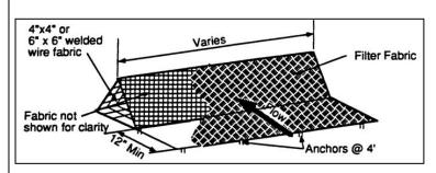
**Description:** A triangular sediment filter dike is a self-contained silt fence consisting of filter fabric wrapped around welded wire fabric and shaped into a triangular cross section. While similar in use to a silt fence, the dike is reusable, sturdier, transportable, and can be used on paved areas or in situations where it is impractical to install embedded posts for support.
