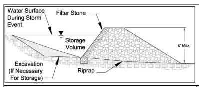
**Description:** A stone outlet sediment trap is a small detention area formed by placing a stone embankment with an integral stone filter outlet across a drainage swale for the purpose of detaining sediment-laden runoff from construction activities. The sediment trap detains runoff long enough to allow most of the suspended sediment to settle while still allowing for diffused flow of runoff.
