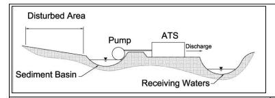
**Description:** An Active Treatment System (ATS) is a small, onsite, water treatment plant used to produce discharge water quality that is better than can be achieved by traditional sediment controls. Common ATS methods are filtration and chemical-aided coagulation/flocculation.
