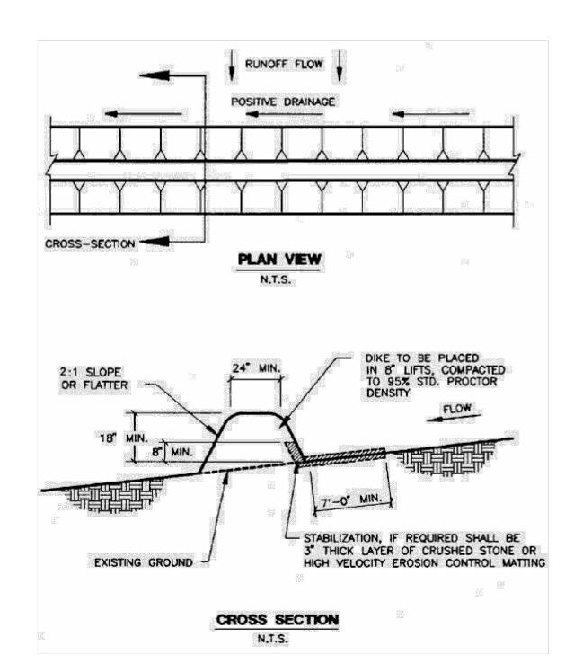
Figure 1-8 Schematic of a Diversion Dike (NCTCOG, 1993b)
