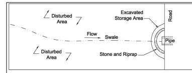
**Description:** The pipe inlet sediment trap is a barrier surrounding a pipe inlet to capture sediment before it enters a closed drainage system. The barrier may be made of concrete block and filter stone or stone riprap and filter stone. The barrier provides both filtration and detention for sediment to settle in the excavated area.
