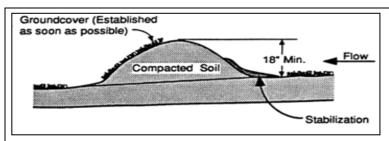
**Description:** A diversion dike is a compacted soil mound, which redirects runoff to a desired location. The dike is typically stabilized with natural grass for low velocities or with stone or erosion control mats for higher velocities.
