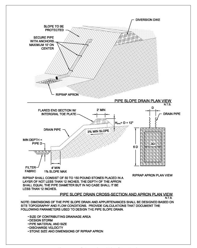
Figure 2.10 Schematics of Pipe Slope Drain
