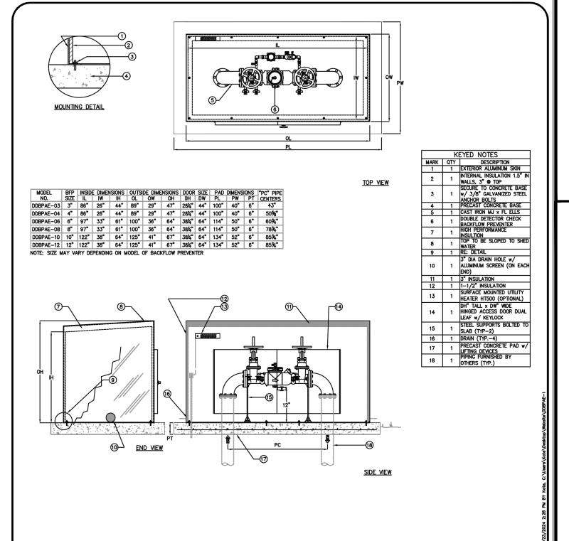
Specifications THE MODEL ERP ALUMINUM ENCLOSURE IS PRE ENGINEERED TO PROVIDE PROTECTION TO BACKFLOW PREVENTERS, METERS, PUMPS, AND OTHER DEVICES INSTALLED ABOVE GROUND. THESE WATER CONVEYING DEVICES ARE SUBJECT TO FREEZING AND VANDALISM. THE ENCLOSURE IS DESIGNED TO BE INSTALLED OVER THE EQUIPMENT AFTER INSTALLATION. THE ENCLOSURE IS EQUIPPED WITH ACCESS DOORS TO PROVIDE ADEQUATE ACCESS TO THE EQUIPMENT. CONSTRUCTION
