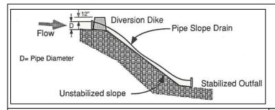
**Description:** A pipe slope drain is a temporary or permanent pipeline, typically utilizing flexible pipe that conveys runoff down steep or unstabilized slopes without causing erosion. The drain is anchored on the upstream end with some form of headwall to limit erosion and secure the pipe.
