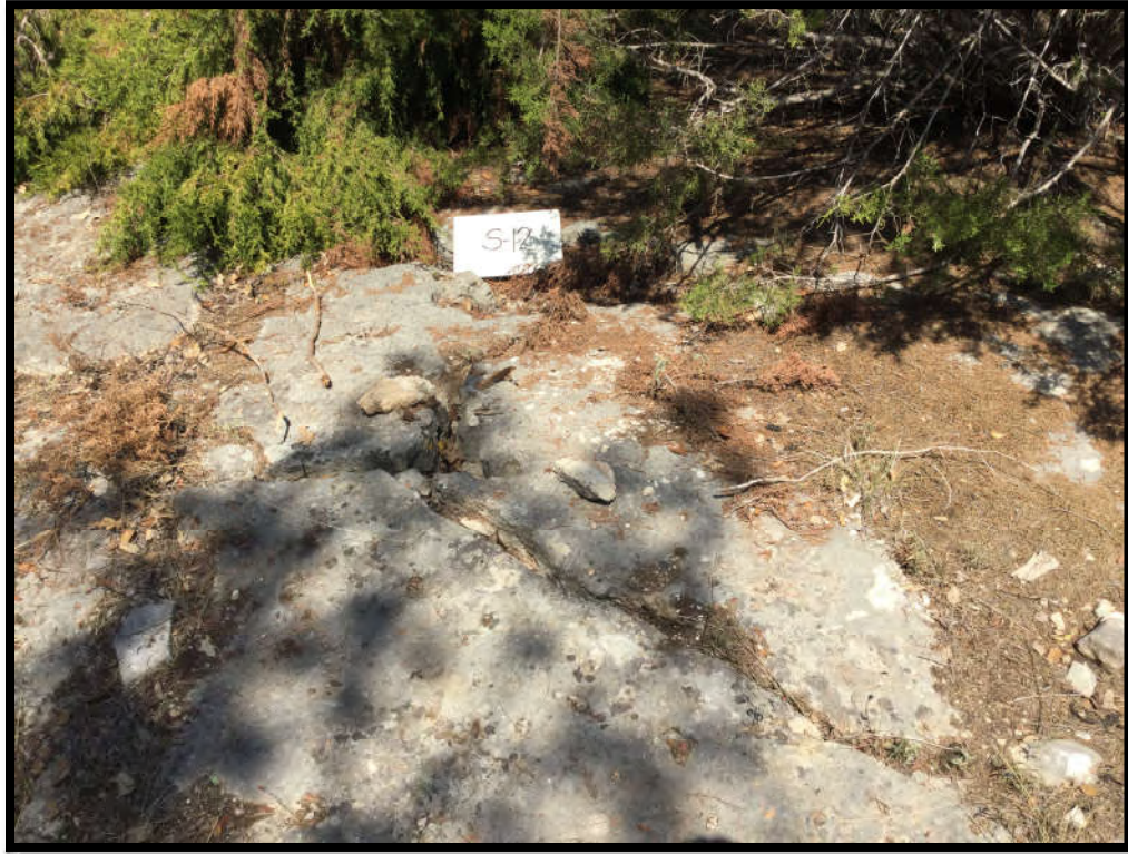
S-12: Solution-enlarged fracture infilled with loose organics.
