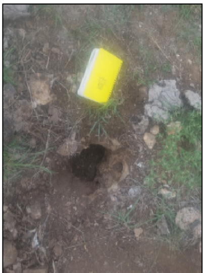
PHOTO 3 View of geologic feature F-2 (solution cavity), facing down
