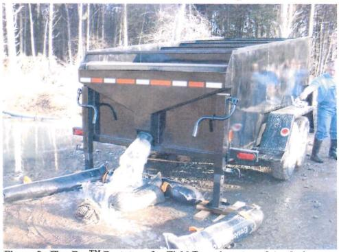
Figure 3. Floc Box<sup>TM</sup> Prototype for Field Experiments and Analysis.
