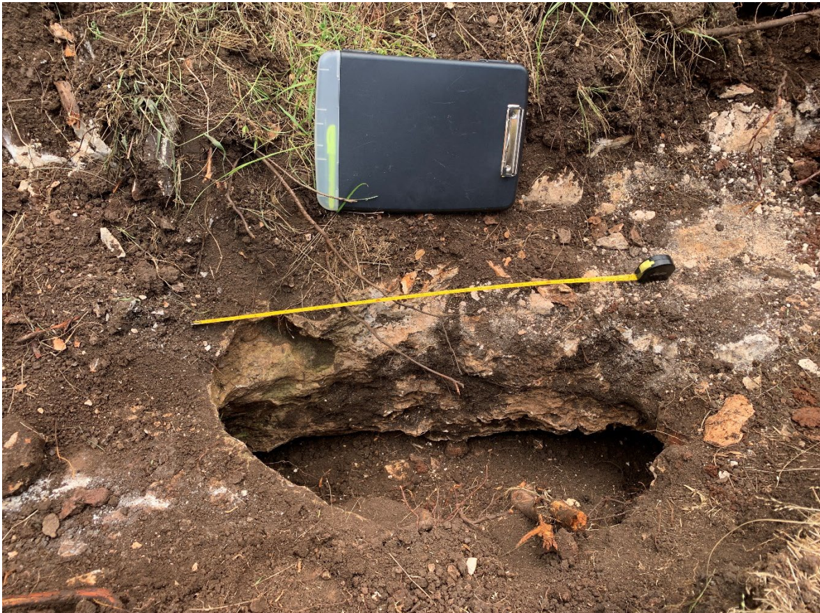
7. S-9 feature cavity (a weathered bedding plane underlies the bedrock overburden)
