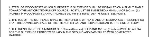
4. SILT FENCE FABRIC SHOULD BE SECURELY FASTENED TO EACH STEEL OR WOOD SUPPORT POST OR TO WOVEN WIRE, WHICH IS IN TURN ATTACHED TO THE STEEL OR WOOD FENCE POST. 5. INSPECTION SHALL BE MADE WEEKLY OR AFTER EACH RAINFALL EVENT AND REPAIR OR REPLACEMENT SHALL BE MADE PROMPTY AS NEEDED.
