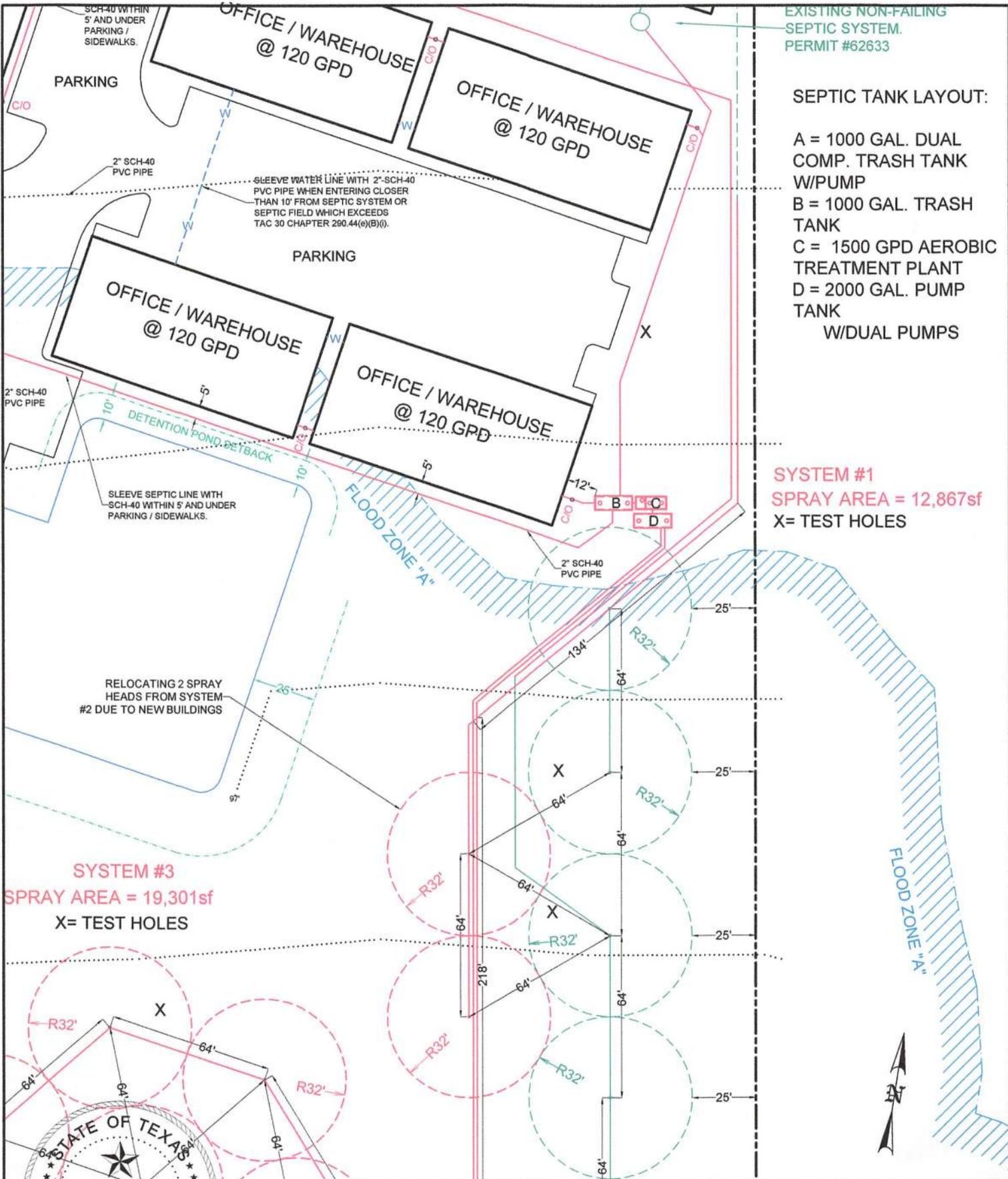
EXISTING NON-FAILING SEPTIC SYSTEM. PERMIT #62633
