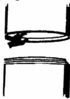
Lubricate bell joint surface liberally, covering entire inside surface using proper pipe gasket lubricant.
