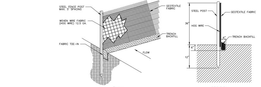
2 SILT FENCE DETAIL N.T.S.
