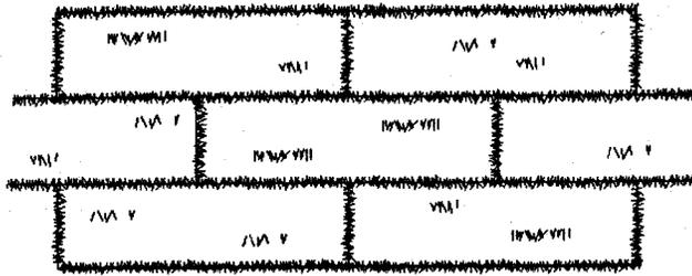
LAY SOD IN A STAGGERED PATTERN. BUTT THE STRIPS TIGHTLY AGAINST EACH OTHER. DO NOT LEAVE SPACES AND DO NOT OVERLAP. A SHARPENED MASON'S TROWEL IS A HANDY TOOL FOR TUCKING DOWN THE ENDS AND TRIMMING PIECES.
