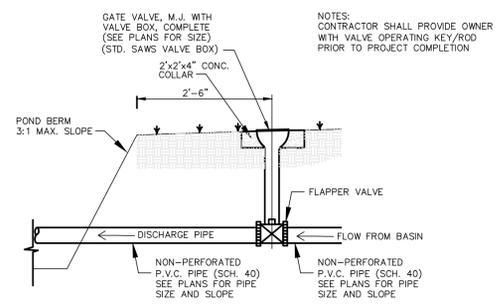
NOTE: VALVE BOX SHALL HAVE WORD "DRAIN" CAST ON COVER.
