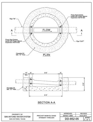
**MANHOLE PLAN AND SECTION A-A**
