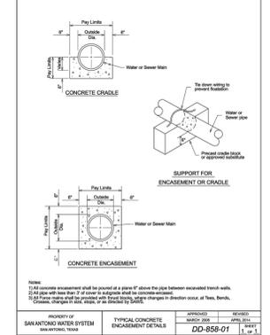
**TYPICAL CONCRETE ENCASUREMENT DETAIL**
