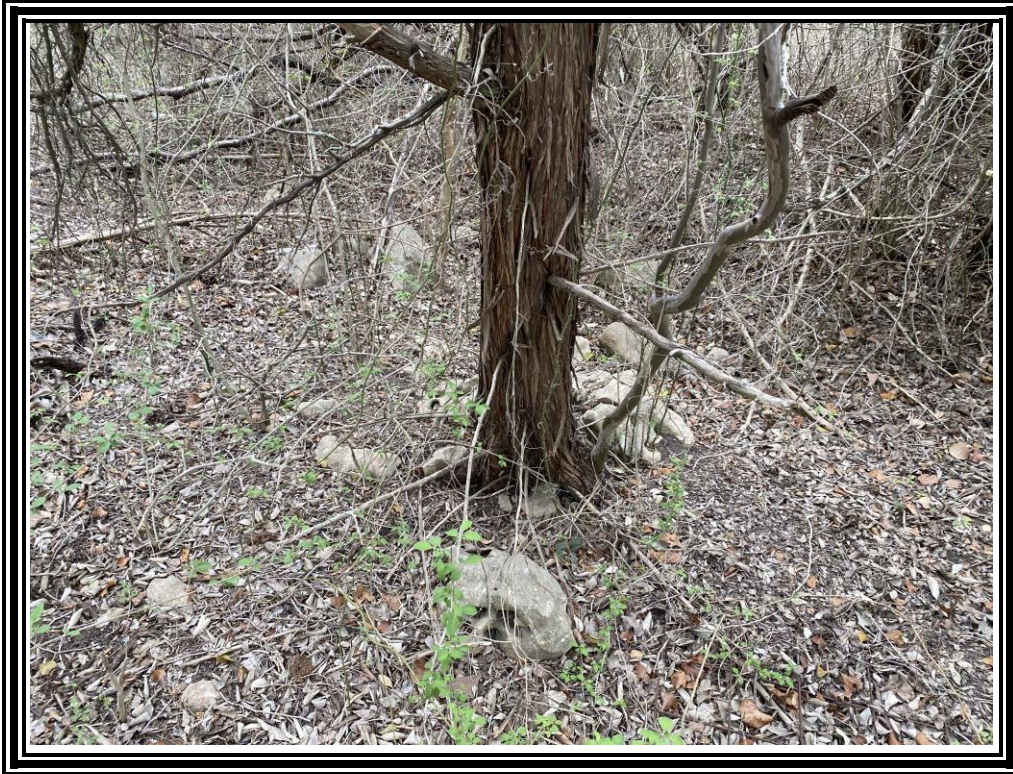
11. View of Georgetown Limestone on the surface in the northwest portion of the site. Geotechnical borings confirmed shallow depths to hard limestones in this area, while areas where the Ilmatogyra Arietina bivalve fossils were seen had thick clay sections in the borings on the east and southeast portions of the site.
