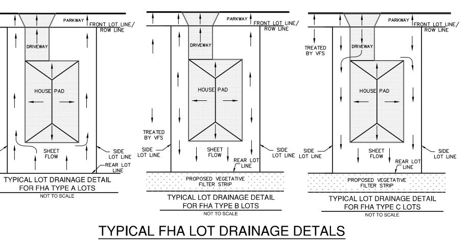
NOTE: ROOF DRAINAGE PATTERN IS APPROXIMATE AND SUBJECT TO CHANGE BASED ON FINAL HOUSE PAD DESIGN. HOWEVER RUNOFF FROM DRIVEWAY, ROOF OR OTHER IMPERVIOUS SURFACES WITHIN THE LOT WILL NOT FLOW ACROSS MORE THAN 72' OF IMPERVIOUS SURFACE BEFORE REACHING THE PROPOSED 15' ENGINEERED VEGETATIVE FILTER STRIP. FINAL LOT GRADING TO ALLOW FOR SHEET FLOW OVER VEGETATIVE FILTER STRIP.
