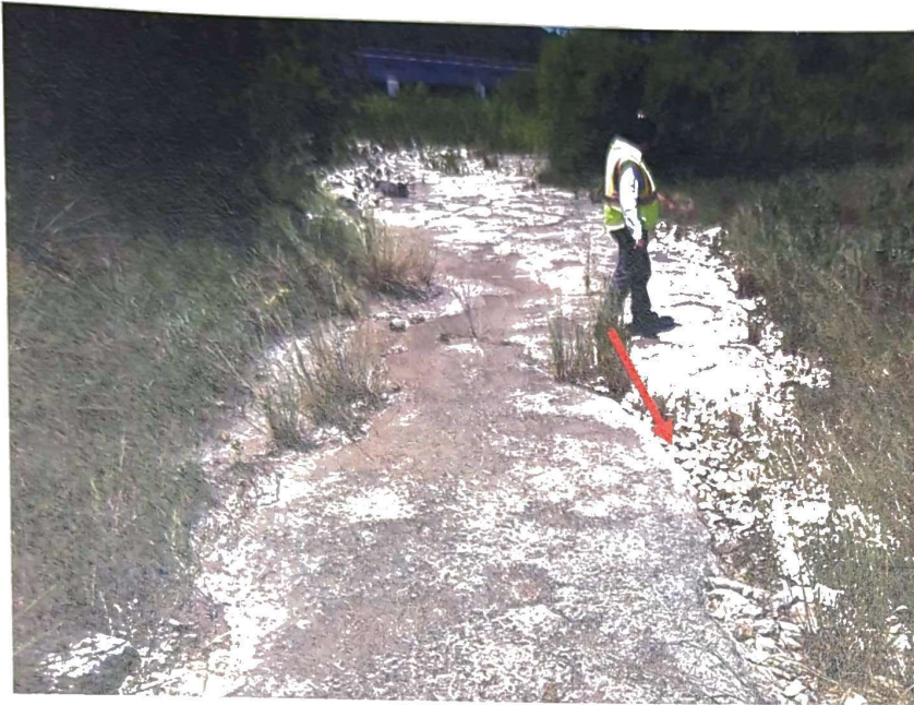
Photograph 9. Solution enlarged fractures were observed in the limestone. The fractures were filled with fine material including gravel, clay, and organics.
