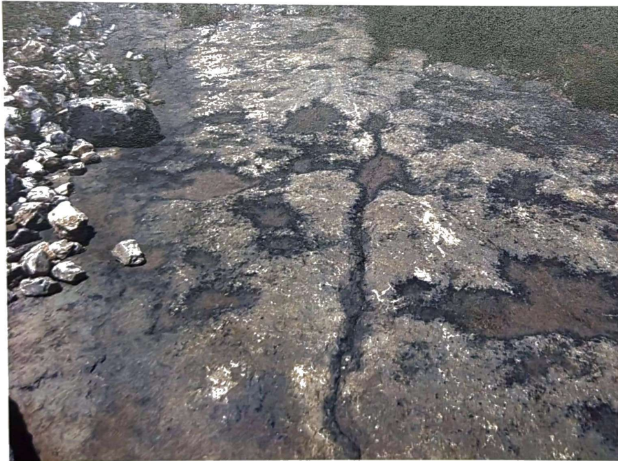
Photograph 9. Solution enlarged fractures were observed in the limestone. The fractures were filled with fine material including gravel, clay, and organics.
