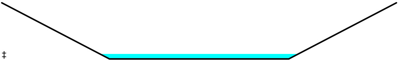
Reach 3R: Grassy Swale
