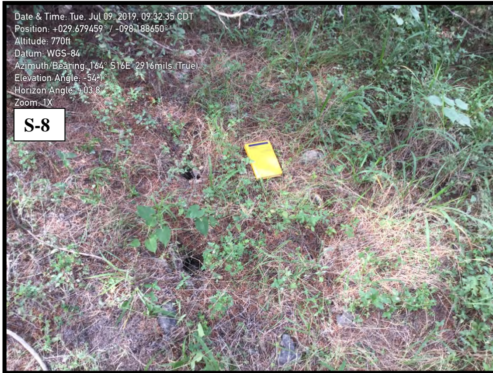
Zone S-8: Clustered and aligned solution cavities
