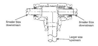
Continuous Monitoring - The Dualoy 3000/LCX system has exceptional performance in continuously monitored systems. Due to its small interstitial space, it is very reliable in detecting leaks in systems monitored by pressure, vacuum or hydrostatic methods. False alarms are eliminated by the lesser sensitivity to external conditions while detection capability of actual leaks is increased. Consult NOV Fiber Glass Systems Engineering for details and design of monitoring methods.
