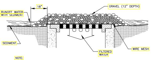
WIRE MESH SHALL BE LAID OVER THE DROP INLET SO THAT THE WIRE EXTENDS MINIMUM OF 1 FOOT BEYOND EACH SIDE OF THE INLET STRUCTURE. HARDWARE CLOTH OR COMPARABLE WIRE MESH WITH 1/2-INCH OPENINGS SHALL BE USED. IF MORE THAN ONE STRIP OF MESH IS NECESSARY, THE STRIPS SHALL BE OVERLAPPED.
