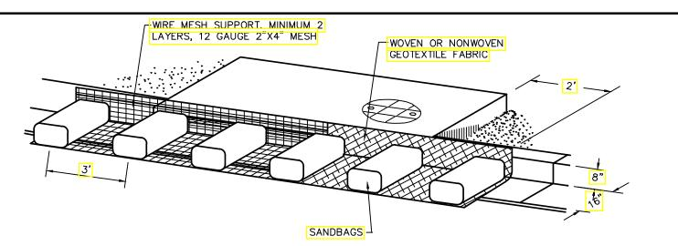
WHEN A SANDBAG IS FILLED WITH MATERIAL, THE OPEN END OF THE SANDBAG SHOULD BE STAPLED OR TIED WITH NYLON OR POLY CHORD.
