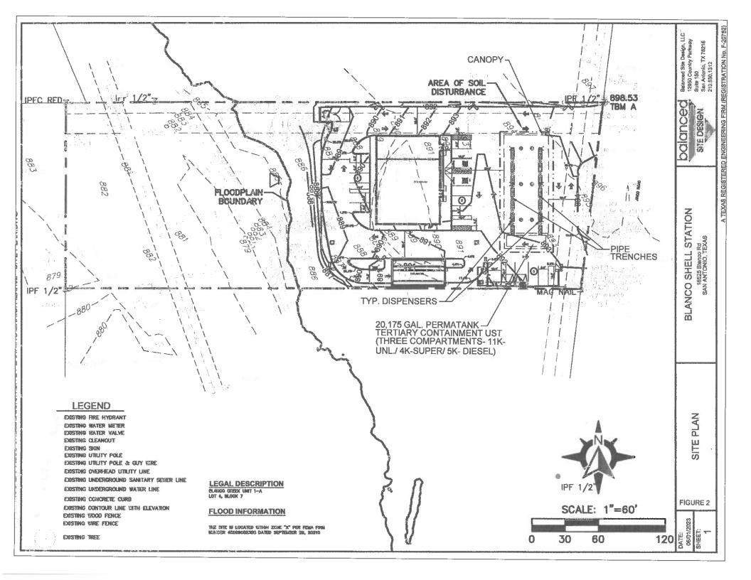
1. THE UST SYSTEM SHALL COMPLY WITH ALL TECHNICAL REQUIREMENTS OF TCEQ CHAPTER 334 SUBCHAPTER C, TECHNICAL STANDARDS 334.41 THROUGH 334.56. THESE TECHNICAL REQUIREMENTS TAKE PRECEDENCE OVER MANUFACTURERS SPECIFICATIONS AND INSTRUCTIONS AND NATIONALLY RECOGNIZED ASSOCIATIONS OR INDEPENDENT TESTING LABORATORY.
