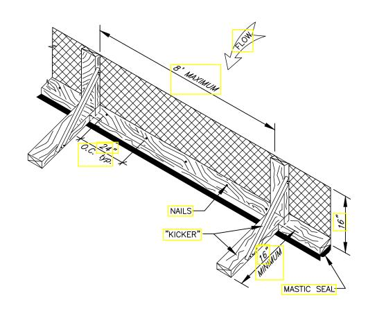
SILT FENCE ON PAVEMENT DETAIL NOT TO SCALE
