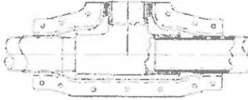
**Size Reductions** - For large systems where larger diameter trunk lines are used, pipe diameter reductions are easily made with the Dualoy 3000/LCX system at fittings. Single piece bushings are used in the primary fitting to reduce the primary pipe size. The containment pipe size is reduced by bonding a 2-piece reducer ring between the clamshell and the smaller pipe jacket. No cutting of clamshell fitting tapers is involved.
