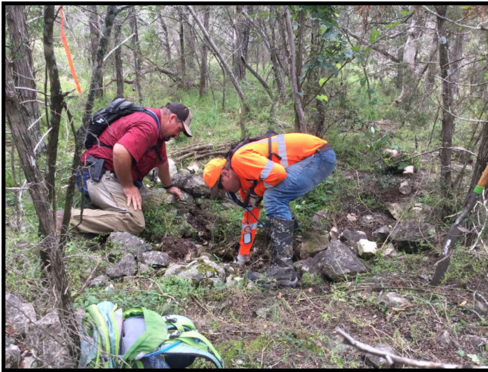
S-27: Hand excavation of loose cobbles of one of the sinkholes that make up this zone feature.
