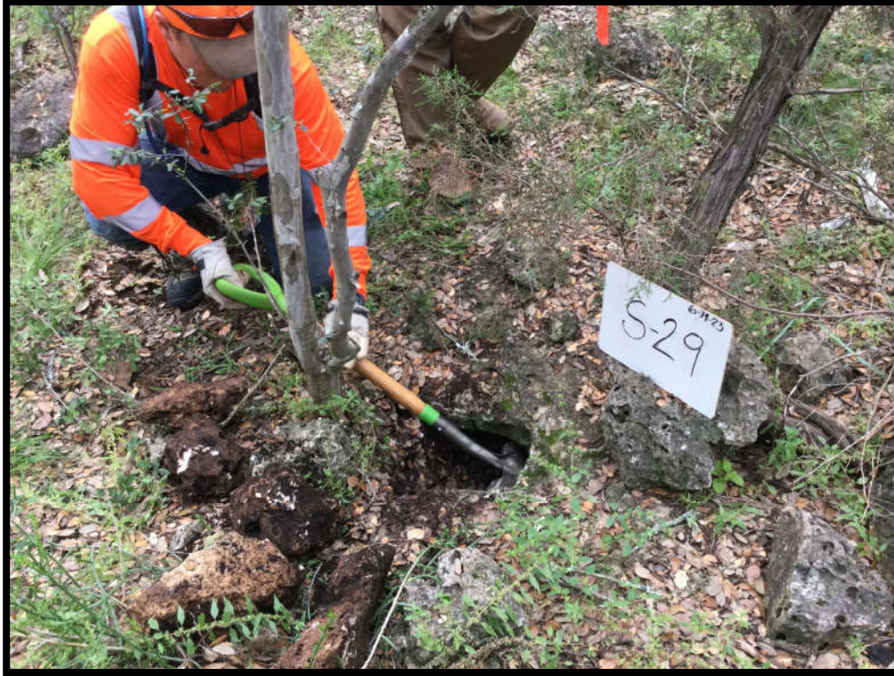
S-29: Hand excavation of one of the solution cavities that make up this zone feature.
