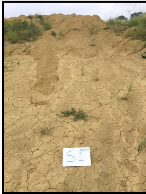
Feature S-1: Floor of closed depression on the southern part of the Site with exposed Kdr.
