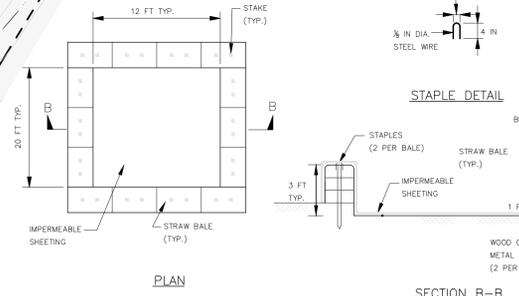
TYPICAL CONCRETE TRUCK WASHOUT PIT
