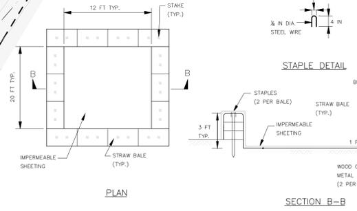
**TYPICAL CONCRETE TRUCK WASHOUT PIT**
