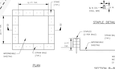
TYPICAL CONCRETE TRUCK WASHOUT PIT
