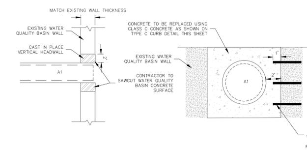
**STORM DRAIN LINE TO WATER QUALITY BASIN CONNECTION DETAIL**
