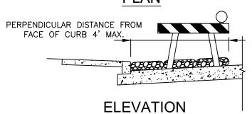
STRADDLE GRAVEL FILTER BAGS WITH TYPE 1 BARRICADES MOUNTED WITH TYPE "A" FLASHING WARNING LIGHT. SEE BARRICADE CONSTRUCTION SIGN DETAILS. PLACE FLASHING LIGHTS AWAY FROM GUTTER. FLUSH WITH OUTSIDE EDGE OF BAG CONFIGURATION.
