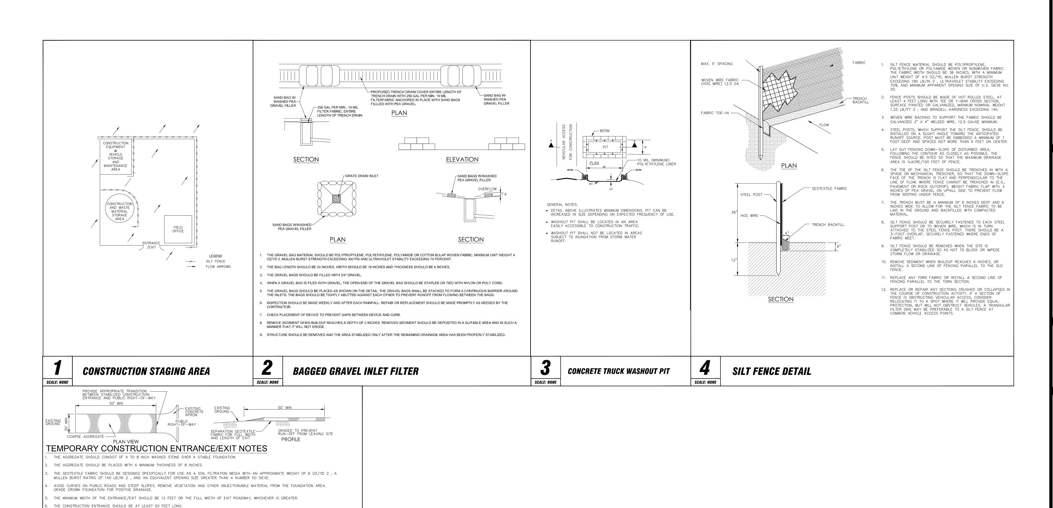
PLACE GEOTEXTILE FABRIC AND GRADE FOUNDATION TO IMPROVE STABILITY, ESPECIALLY WHERE WET CONDITIONS ARE ANTICIPATED.
